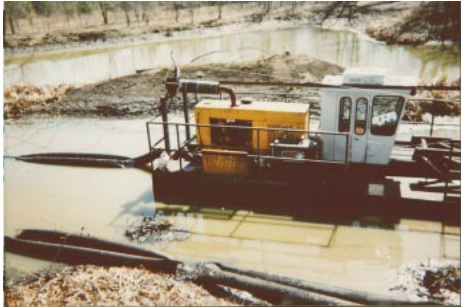
A barge pumps waste from an on-site lagoon at the National Presto Industries site, Eau Claire, Wis.
