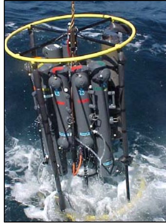
Water testing equipment collects samples for on-board analysis
