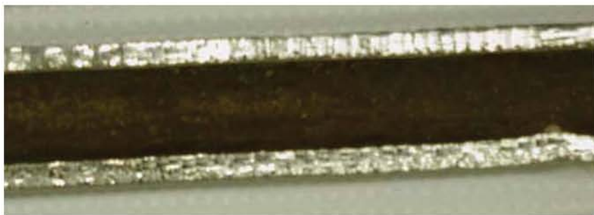
Inside of lead service line extracted from DC water system
