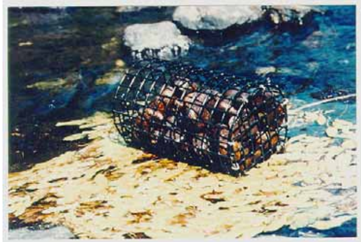
FIGURE 6-1. Rock-filled wire basket used as introduced substrate.
