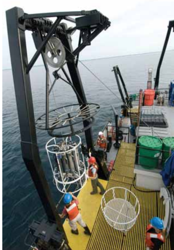
Launching the Rosette Water Sampler from the R/V Lake Guardian
