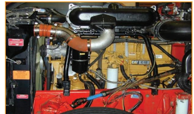
Membranes within the black housing mounted over the diesel engine pictured above generate NEA from cooled turbocharged air.
