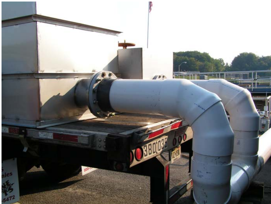
Figure 3-2. Influent (top) and effluent (bottom) piping configuration for the V-40R-A150 test unit channel.
