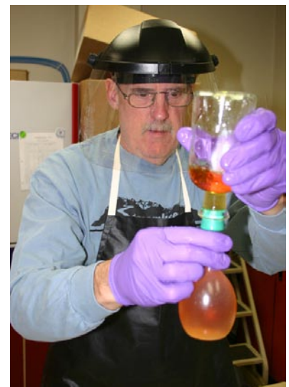
Volunteer Steve Belcher prepares a Winkler titration to use in monthly accuracy checking of dissolved oxygen meters.
