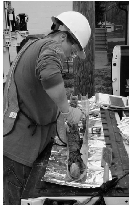
A contractor prepares a soil boring for laboratory analysis.
