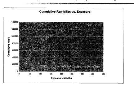
Figure 1: Non-Scrap-Adjusted Mileage Model
