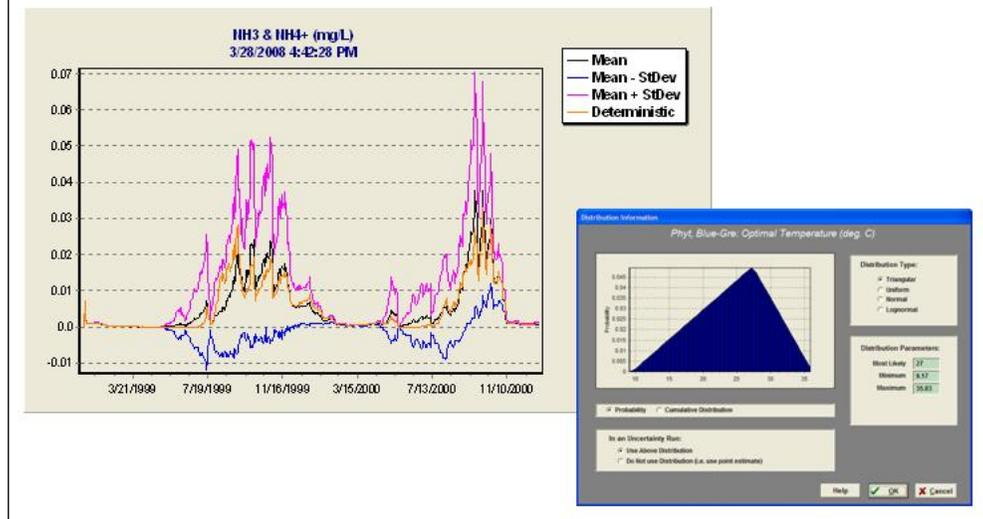
Input utilizes a graphical interface with several possible distributions for each of the loadings or parameters being tested. Output includes graphs of the deterministic, mean,  $\pm 1$  standard deviation, maximum, and minimum values. Output can also be shown as a biomass risk graph (see slide 171). Furthermore, output for each iteration of the analysis can be saved as csv files (in Release 3.1).
