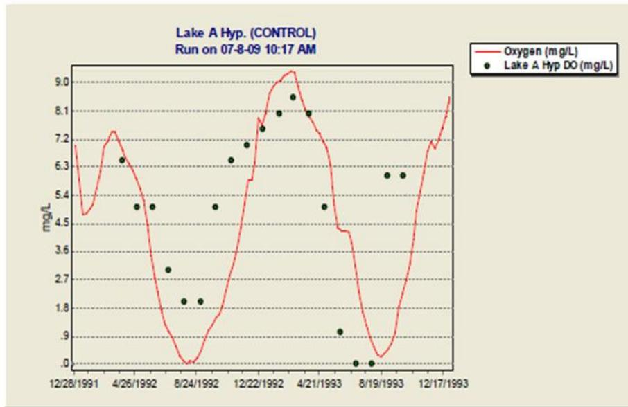
The sediment diagenesis submodel was necessary to represent the influence of bottom sediments on hypoxia.
