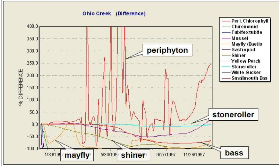
The best indication of the impacts are to be seen in a **Difference** graph that compares the perturbed with the control. To get this you have to run the simulations for the same period. Note that most of the invertebrates disappear quickly, followed by the fish. Shiners and stonerollers share the same toxicity record (“Minnow”), so the relative decline of shinners is due to loss of invertebrate food base and not direct toxicity whereas stonerollers, which graze periphyton, are unaffected.
