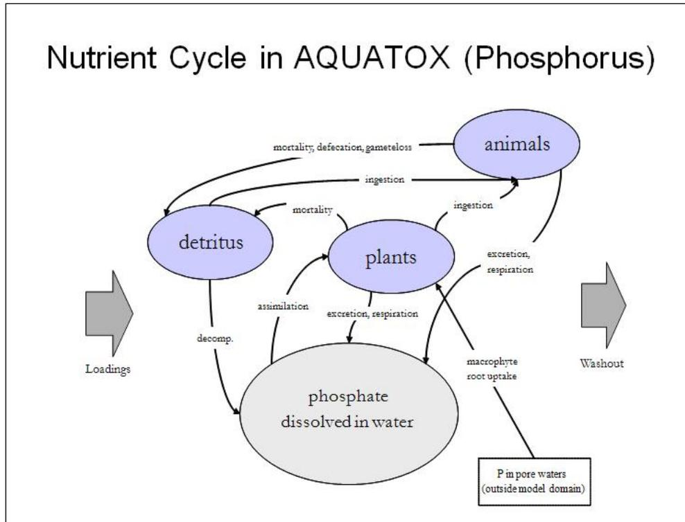
In addition to the pathways shown, Release 3 can simulate precipitation of  $\text{CaCO}_3$  with sedimentation of sorbed P.
