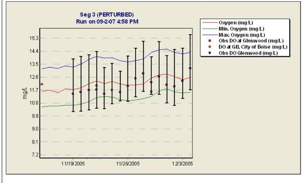
Predicted and observed diel dissolved oxygen at Glenwood Bridge, Lower Boise River, Idaho. This is applicable during low-flow when photosynthesis is dominant within the reach. However, during high flow the DO is completely dominated by loadings from upstream. You should always check the retention times for a particular reach.
