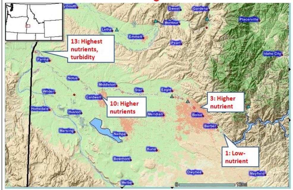
The Lower Boise River is a shallow river that is heavily managed for irrigation. In fact, the downstream segment 10 has the lowest flow because of diversions; below that reach, drains bring in nutrient- and sediment-laden return flow.
