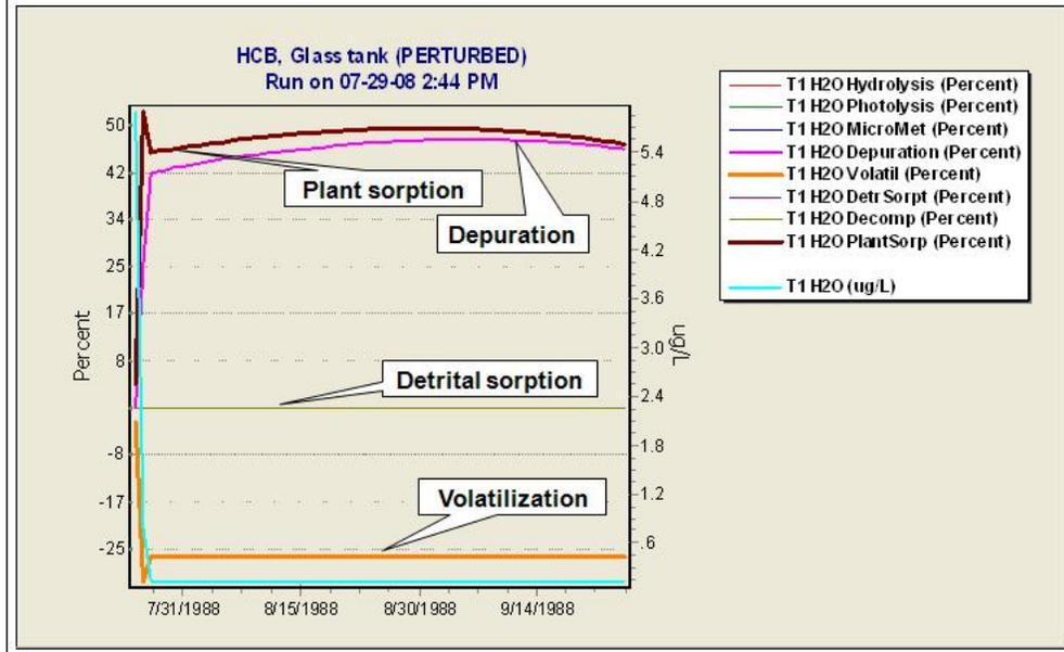
The rates plot indicate that the only significant processes in the tank are sorption by plants and volatilization. As we saw on the previous slide, the rate of sorption by detritus is almost the same as for plants; however the amount of detritus is so small that it accounts for only a fraction of a percent of the HCB in the water. The macrophytes, on the other hand, have a very large biomass in the tank, so much of the mass of HCB is taken up by the plants.
