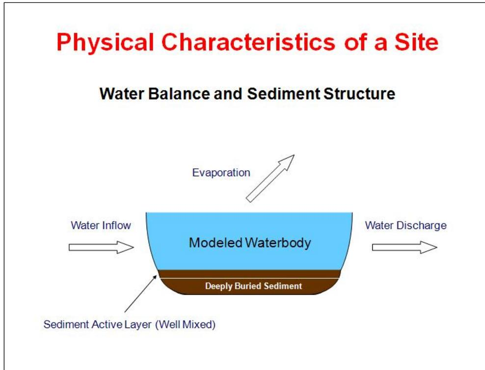
Water balance is defined as a function of inflow, evaporation, and discharge. We will discuss the various mechanisms for modeling water balance in a future slide. The modeled waterbody or river segment is assumed to be well mixed. Evaporation is a function of the site's surface area and the mean annual evaporation at the site.
