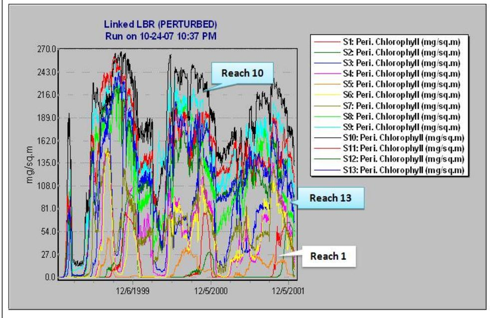
Nutrient-poor Reach 1 has the lowest periphyton biomass. Reach 10 with nutrient-rich clear water has the highest periphyton.
