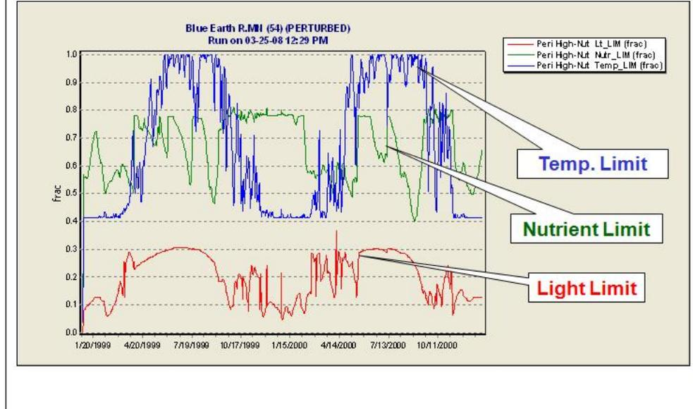
Light limitation means that the plant photosynthesis rate is less than one third of the P<sub>Max</sub>. The temperature limitation reduces photosynthesis during winter months.
