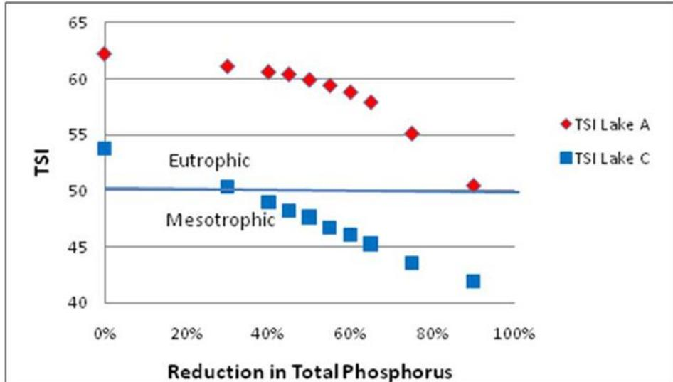
The Trophic State Index, TSI, based on chlorophyll is a useful way of presenting the results in the context of a eutrophication gradient. The simulated TSI values exhibit a gradient toward the dam during the 1992-93 period. This slide shows the predicted responses of both Lacustrine A and C to load reductions. A 30% reduction in TP loads places Lacustrine C on the borderline between eutrophic and mesotrophic, whereas a 90% reduction would be required for Lacustrine A based on the growing season.
