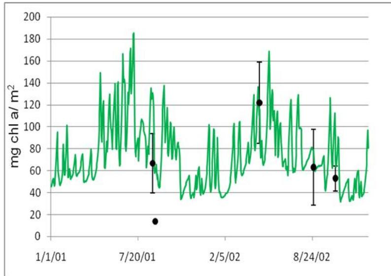
The MN parameter set was used with only a couple modifications. The critical force for periphyton scour was increased based on the bedrock riffles, and the optimum temperature was increased for two groups based on the difference in temperature between MN and AL. Therefore, this is considered a good partial validation.
