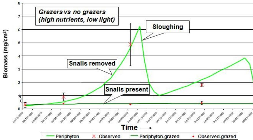
This graph was the result of a model validation exercise utilizing a comprehensive dataset from a series of experiments that manipulated nutrient levels, ambient light and grazing pressure by snails (Rosemond, 1993). The model was calibrated using the experimental results, and then validated against ambient stream conditions. Two simulations illustrate the importance of grazing and sloughing.
