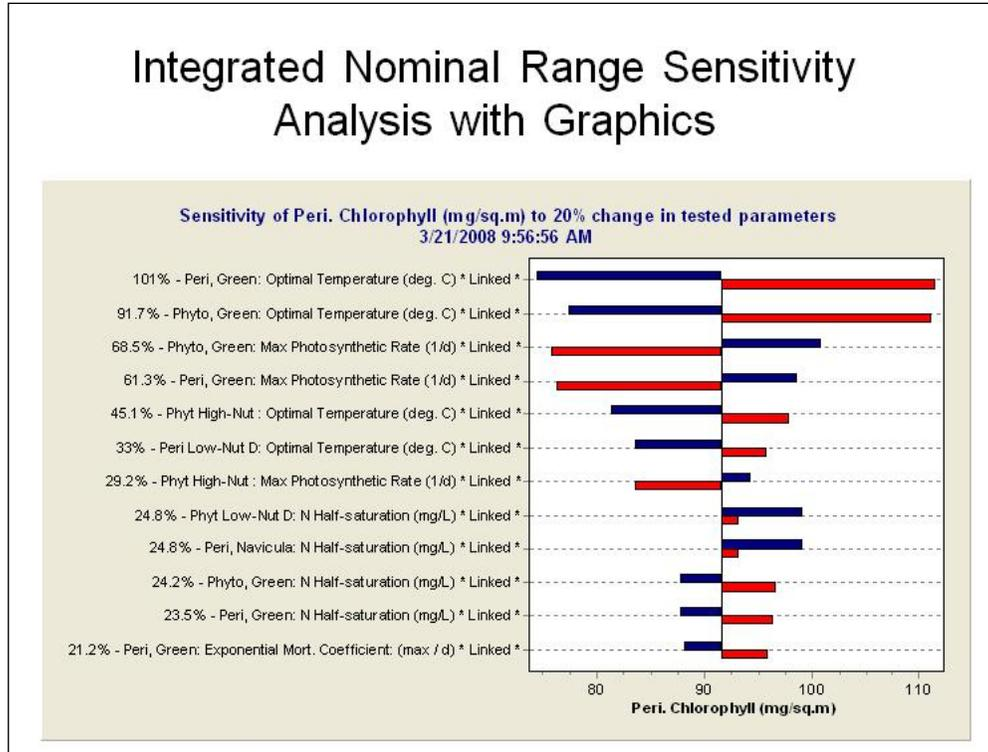
AQUATOX can automate a nominal range sensitivity analysis (also known as a "one-at-a-time" sensitivity analysis), in which multiple parameters are changed by a given percentage. The sensitivity of model output to the different perturbations can then be compared.
