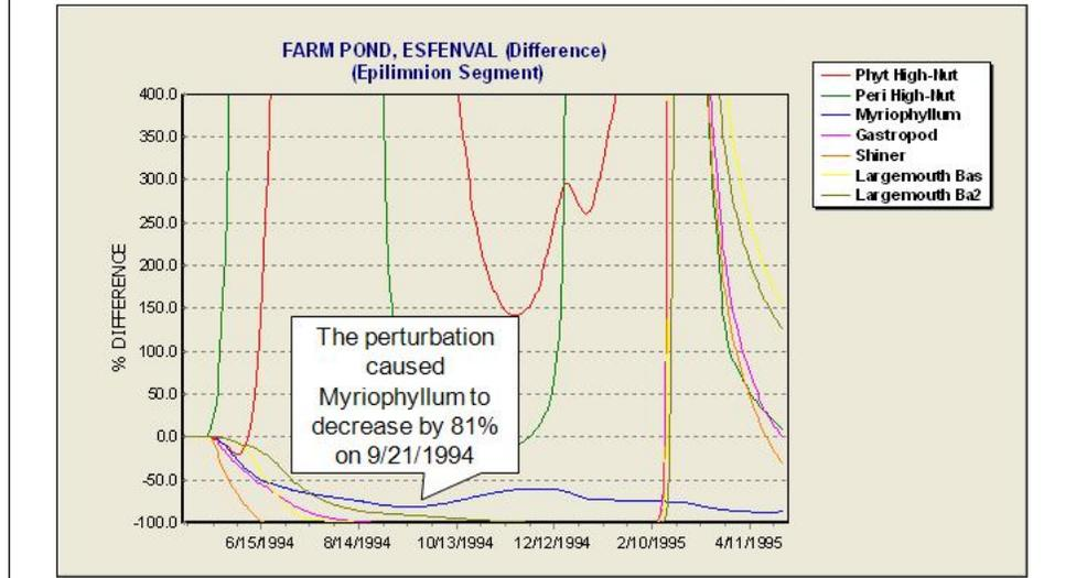
The equation shown calculates the percent difference that the perturbation (in this case, addition of esfenvalerate) causes from the control simulation. By this formulation a 100% difference means that the perturbation caused the state variable to double. A negative 50% difference means that the perturbation caused the state variable to halve.
