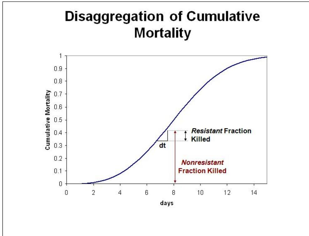
The biomass killed per day is computed by disaggregating the cumulative mortality. Think of the biomass at any given time as consisting of two types: biomass that has already been exposed to the toxicant previously, which is called *Resistant* because it represents the fraction that was not killed; and new biomass that has formed through growth, reproduction, and migration and has not been exposed to a given level of toxicant and therefore is referred to as *Nonresistant*.
