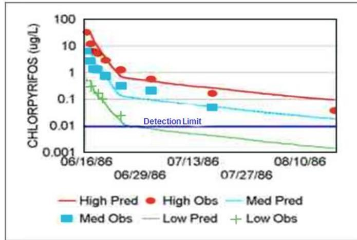
In a validation study several years ago, three levels of chlorpyrifos in a pond were predicted and compared to observed data.
