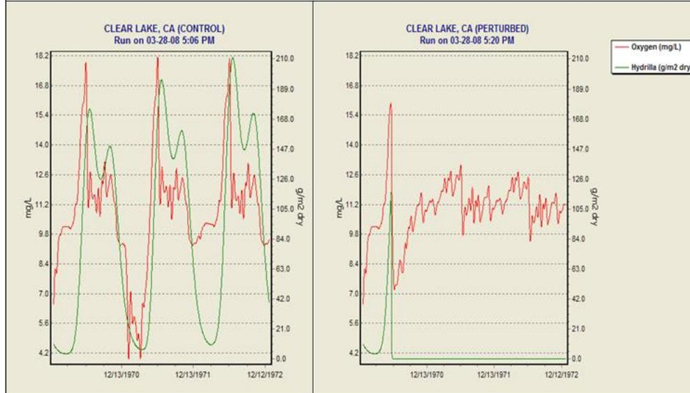
Death of *Hydrilla* due to the fluridone is not predicted to have serious impact on dissolved oxygen. Production of detritus by *Hydrilla* is predicted to impact DO more with seasonal dieoff.
