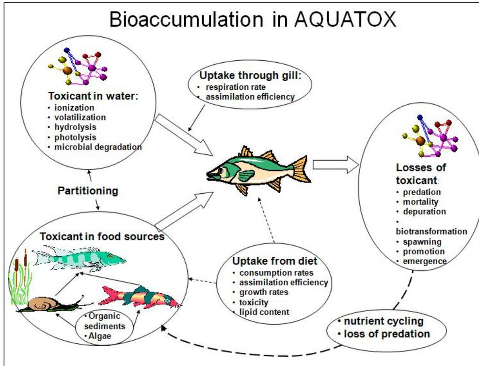
Nonequilibrium concentrations, as represented by kinetic equations, depend on sorption, desorption, and elimination as functions of the chemical and exposure through water and food as a function of bioenergetics of the organism.
