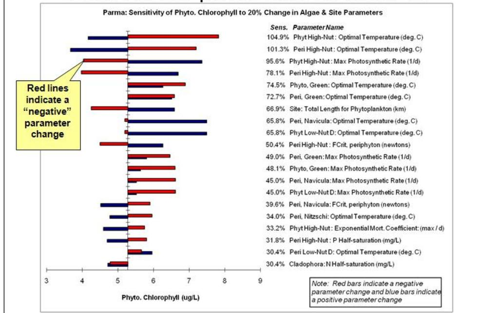
Nominal range sensitivity analysis can be performed easily with AQUATOX. With it you can identify those parameters that make the specific model output most sensitive; this indicates a need for the best data possible for those parameters.
