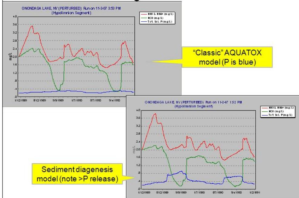
These images are for Onondaga Lake, NY. The diagenesis submodel also had a dramatic effect on the modeling of sediment oxygen demand from the Tenkiller Lake OK sediments. It was nearly impossible to calibrate dissolved oxygen in the Tenkiller hypolimnion without the diagenesis submodel, but with the submodel the simulation calibrated without much effort.
