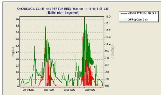
At high pH  $\text{CaCO}_3$  comes out of solution, precipitates, and takes  $\text{PO}_4$  along with it. This process is mediated by algae, so precipitation parallels photosynthesis (shown here as Gross Primary Production).
