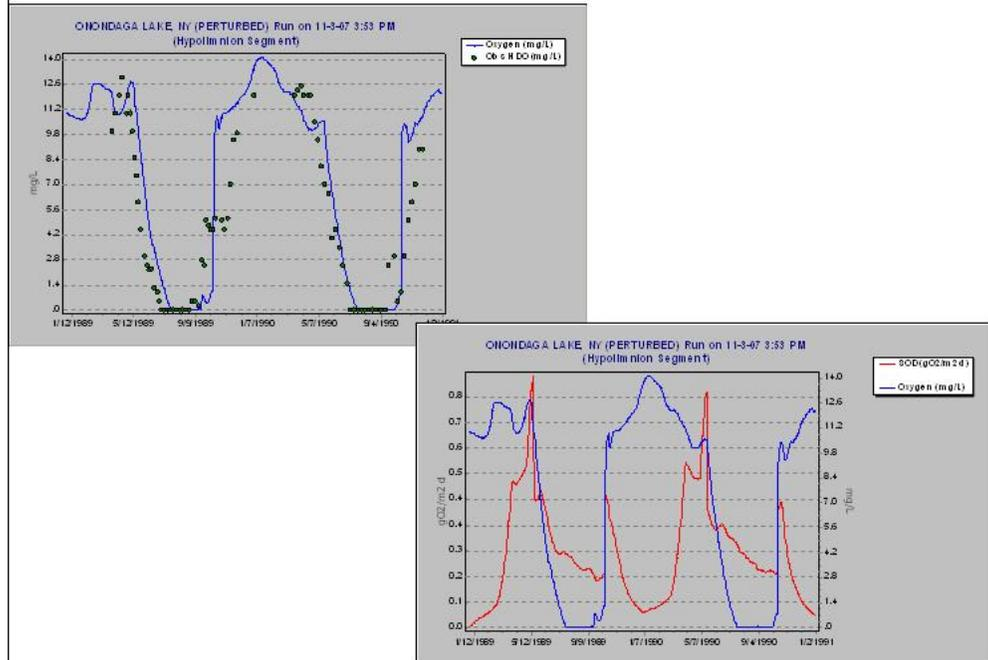
Observed data are shown as circles in the above graph while the AQUATOX simulation is the blue line. Simulated sediment oxygen demand is shown in red.
