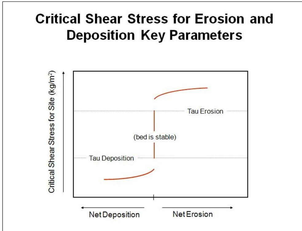
These two parameters are specified for silt and clay and can be found in the Stream section of the Site underlying data. This section of model is identical to HSPF. These parameters can be highly site-specific and are usually used as calibration parameters when calibrating the HSPF inorganic sediment model.
