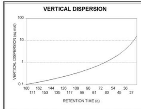
Diffusion between the epilimnion and hypolimnion is a function of the temperature differential. The user specifies the temperatures (or mean and range) for each layer and the model computes when stratification occurs and how much turbulent diffusion occurs.
