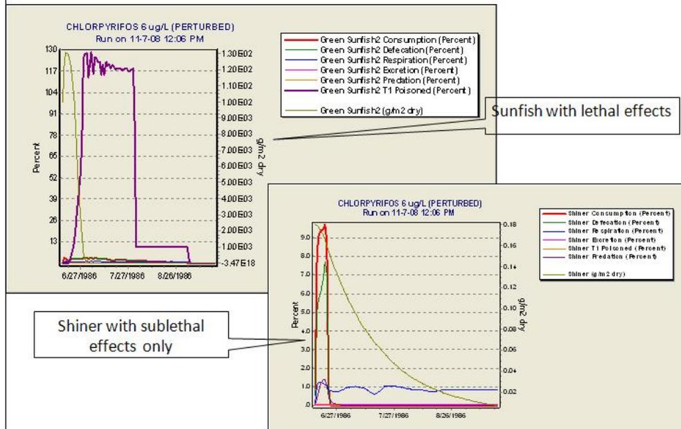
Sunfish have a low tolerance to chlorpyrifos ( $LC_{50} = 2.4 \text{ ug/L}$ ), so bioaccumulation is followed by significant mortality with gradual recovery.
