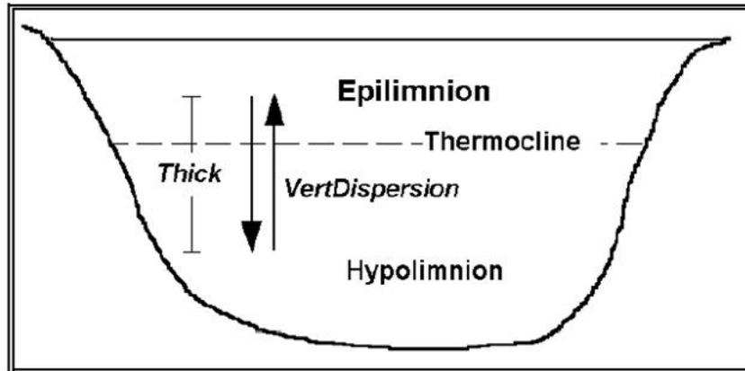
Thermal stratification is handled in the simplest form consistent with the goals of forecasting the effects of nutrients and toxicants. Lakes and reservoirs are considered in the model to have two vertical zones: epilimnion and hypolimnion; the metalimnion zone that separates these is ignored. Instead, the thermocline, or plane of maximum temperature change, is taken as the separator; this is also known as the mixing depth (Hanna, 1990).
