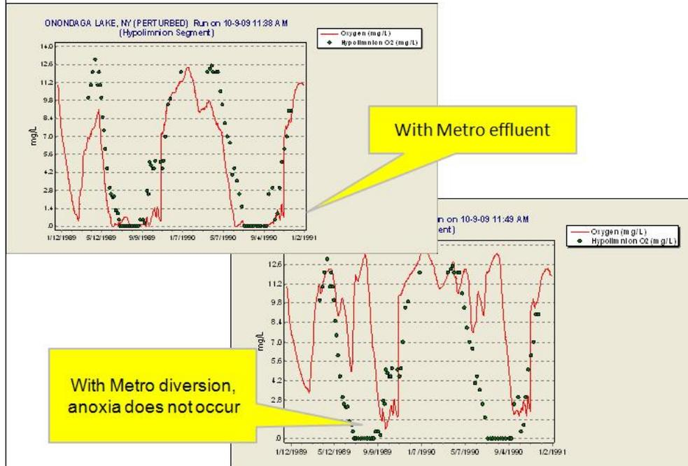
For example, what might be the effects on dissolved oxygen be if the highly nutrient-enriched WWTP discharge into Onondaga Lake were eliminated (one possible management option)? AQUATOX predicts a significant decrease in the magnitude and duration of the hypoxia.
