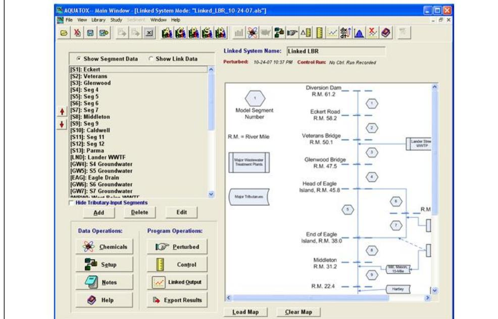
In this example main-stem reaches, tributary agricultural drains, groundwater, and waste water treatment effluents are linked in simulating 61 miles of the Lower Boise River, Idaho.
