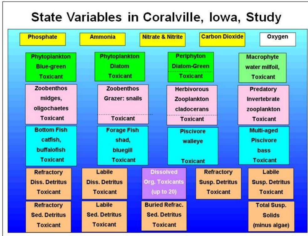
Here is an example of a typical set of compartments used in simulating a eutrophic reservoir. The model can represent complex food webs with ease. Up to 20 organic toxicants can be simulated; however, a toxicant is associated with each compartment, so the total number of state variables may be quite large, slowing down the simulation.
