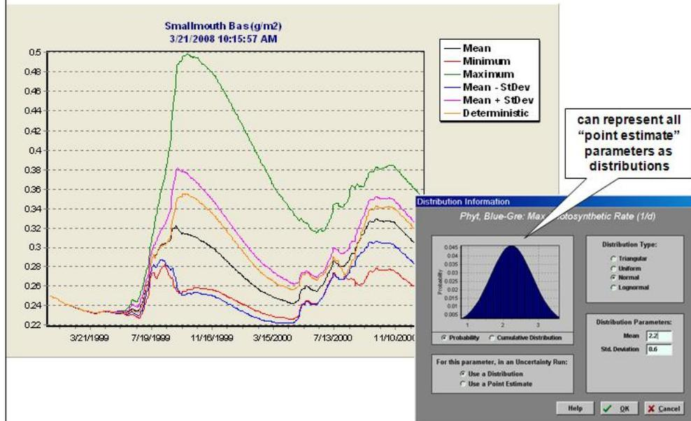
These model results represent summary statistics for each time-step of the simulation based on the Monte-Carlo analysis. The deterministic line plotted represents a single scenario run with “point estimate” values replacing each distribution. All other lines are statistics derived from all of the scenarios run during the analysis.
