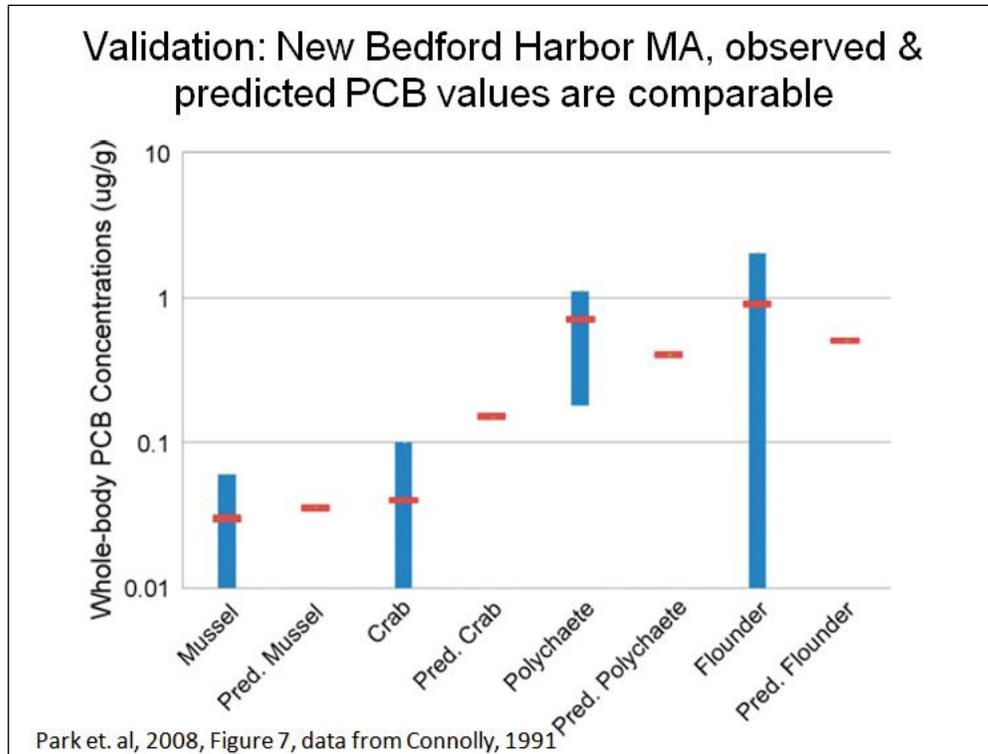
In a partial validation, PCB concentrations in water and sediments in New Bedford Harbor, MA, were imported into Galveston Bay TX simulation. The results were comparable between observed and predicted mean whole-body concentrations.
