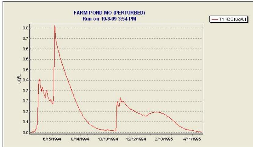
The assumptions in setting up this hypothetical case is that it is a typical farm pond located adjacent to and receiving runoff from a corn field in Missouri. The Pesticide Root Zone Model (PRZM) was run to obtain loadings for AQUATOX using the worst-case scenario out of 20 years (rain with runoff immediately after pesticide applications).
