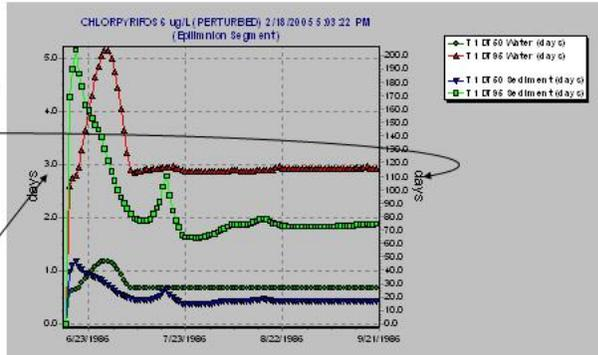
AQUATOX estimates half-lives (DT50s) and time to 95% chemical loss (DT95s) independently in bottom sediment and in the water column. Estimates are produced at each output time-step depending on the average loss rate during that time-step in that medium.
