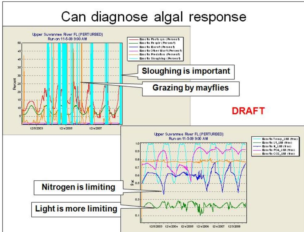
The pH in the Upper Suwannee is low enough that gastropods are excluded, decreasing the herbivory on periphyton. Sloughing, especially when biomass builds up and algae are stressed, is predicted to be an important loss term for this diatom. Total nitrogen (TN) averages 1.48 mg/L; however, much of it is tied up in refractory dissolved organic matter so that N is severely limiting, as is light.
