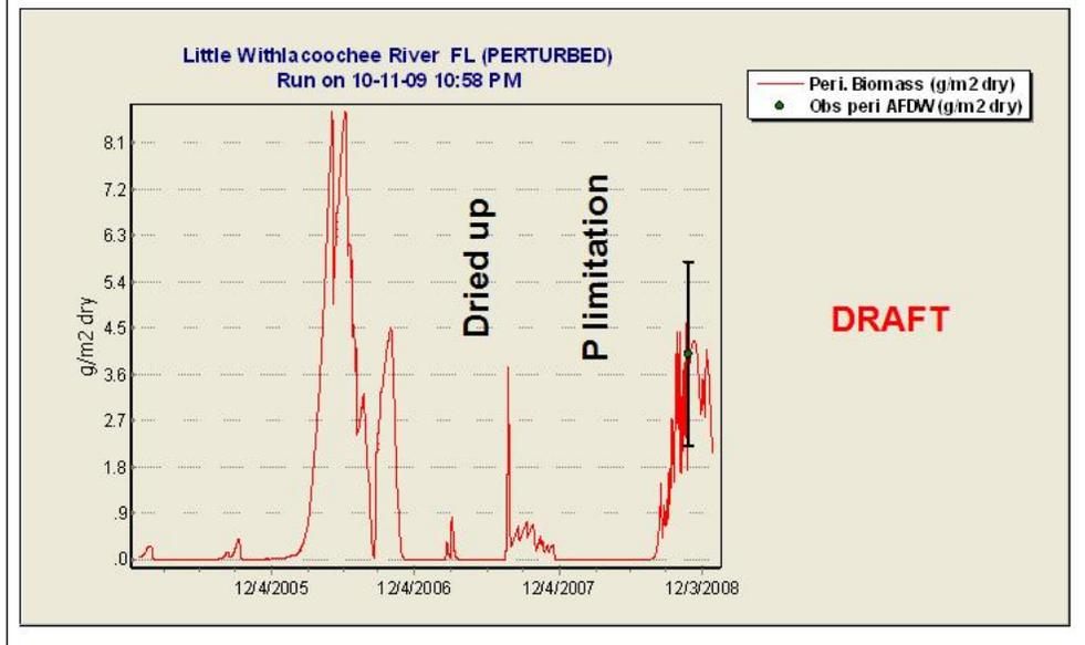
AQUATOX successfully stepped through a period in which the river went dry. Severe phosphorus limitation is predicted to exclude periphyton at times.
