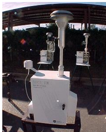
PM 2.5 sampler. The EPA's regulations establish criteria for probe/inlet heights and distance from roadways and other objects. (EPA photo)
