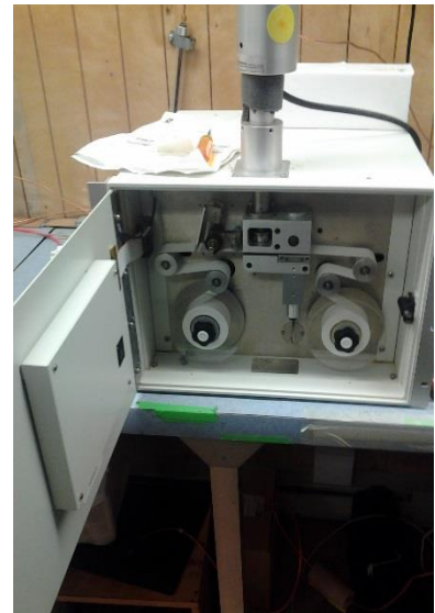
Continuous PM 2.5 monitor, the Beta Attenuation Mass Monitor 1020, in use at the Air Research Station at the EPA campus in Research Triangle Park, North Carolina. (OIG photo)
