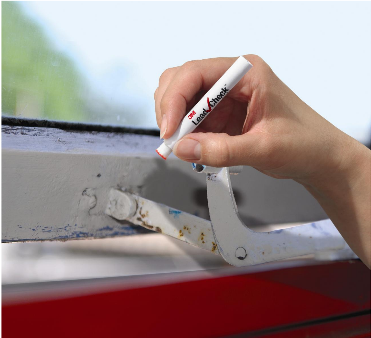
Figure 2-2. 3M™ LeadCheck™ Swabs in Use
