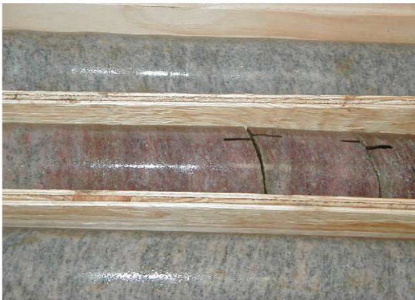
Reddish discoloration noted in R2
