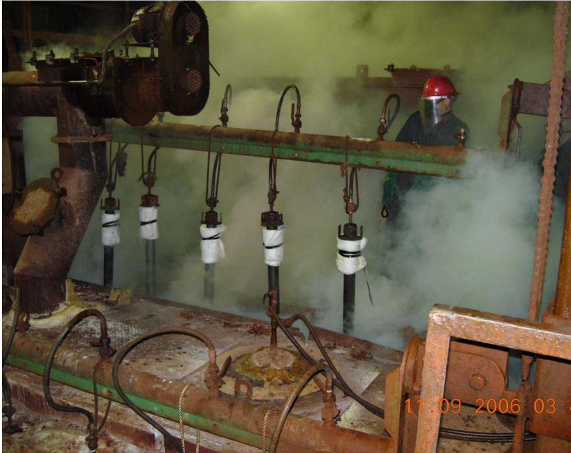
PHOTOGRAPH 23 MR. DERRIC SMITH-MELT REACTOR DUST AND CHLORINE EMISSIONS AS LANCES ARE LOWERED INTO MELT CELL PHOTOGRAPH TAKEN NOVEMBER 9 2006
