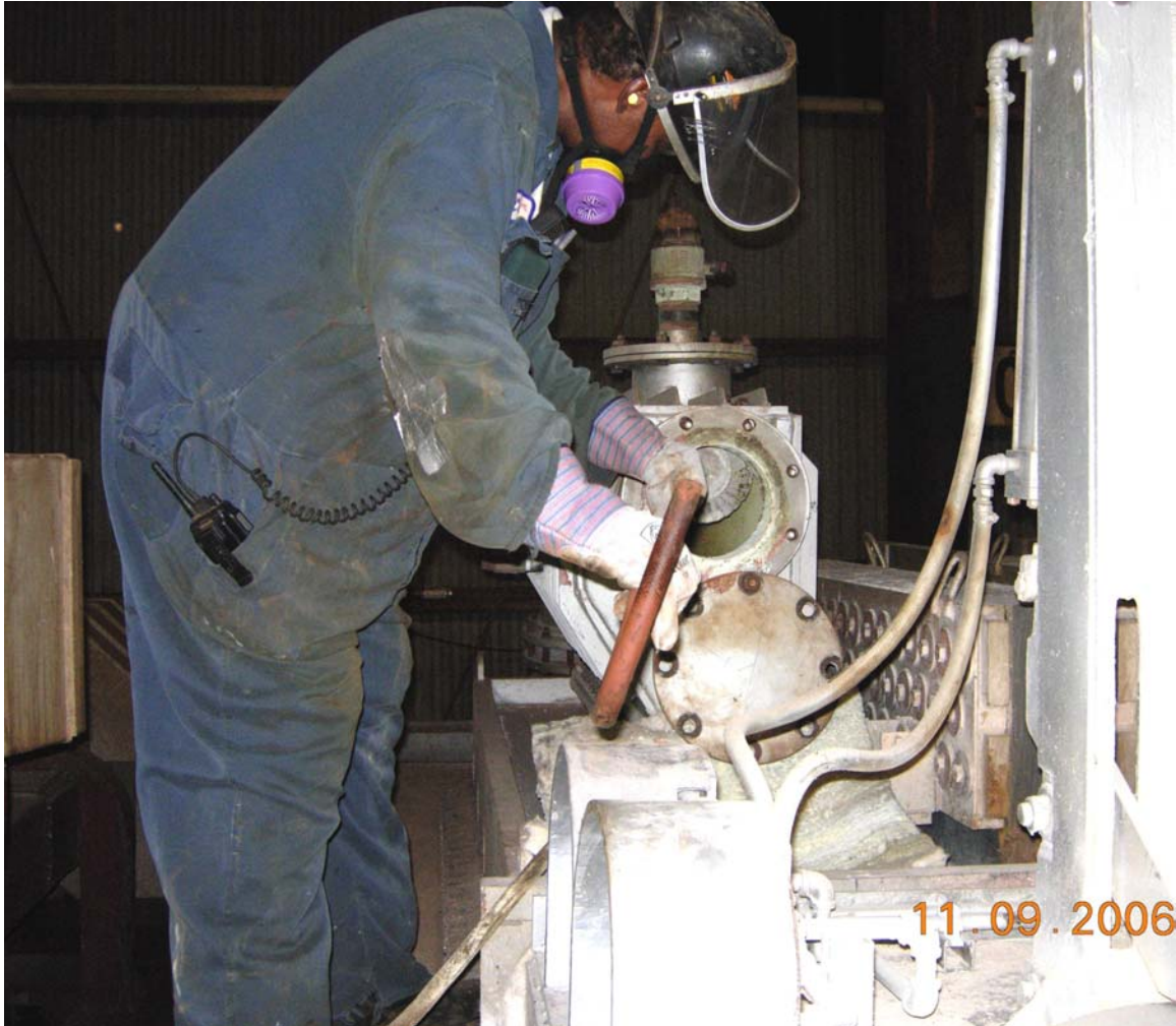
PHOTOGRAPH 21 MR. CARL BURNETT CLEANING ANODE DUST EMISSION FROM THE ELECTROLYTIC CELL COOLING BOX PHOTOGRAPH TAKEN NOVEMBER 9 2006
