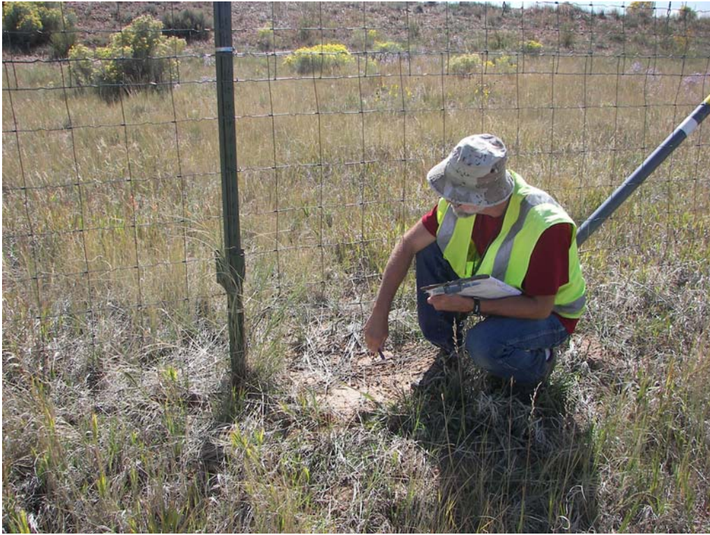
5. One of two holes discovered in the Pond 4 security fence.
