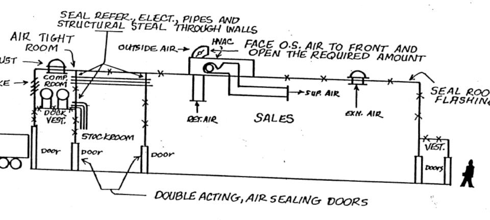
X = SEALED WALLS AND ROOF FLASHINGS
