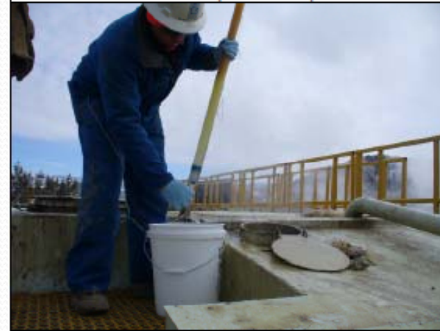
Collecting flowback sample from frac tanks using a bailer
