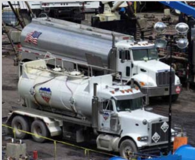
Transport trucks for water (above) and hydraulic fracturing acid (HCl) (below)
