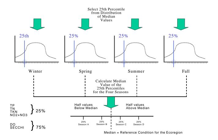
Figure 4b. Illustration of reference condition calculation.
