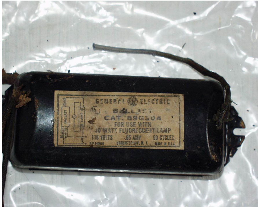
Fig. 4 Fluorescent Light Ballast
