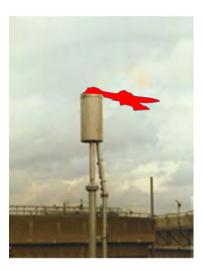
The following image represents a flame below the plane of the exit of the flare tip and attached to the tip. However, since the flame is not discontinuous, this image would not represent Discontinuous Wake Dominated Flow.
