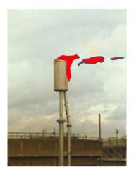
The following image represents a flame below the plane of the exit of the flare tip. However, since the flame is not discontinuous and not immediately adjacent to the tip, this image would not represent Discontinuous Wake Dominated Flow.
