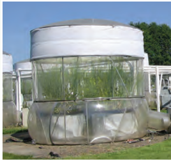
above: Pollen Confinement Chambers are one of the tools used for gene flow studies at Western Ecology Division (WED)
