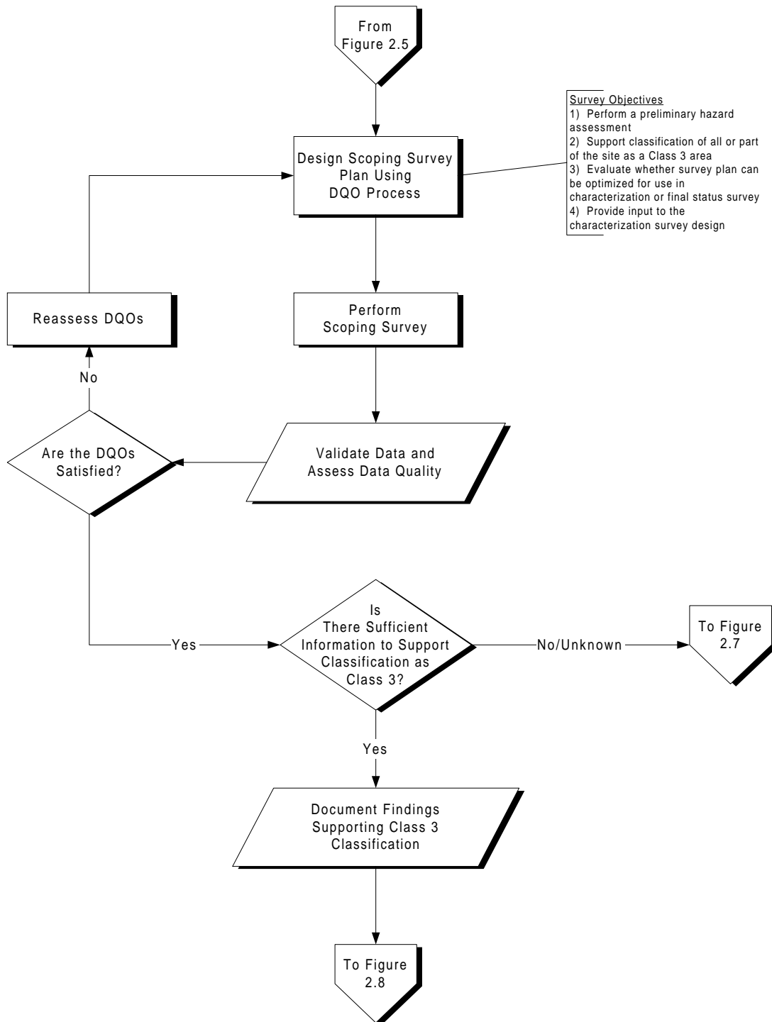
Figure 2.6 The Scoping Survey Portion of the Radiation Survey and Site Investigation Process
