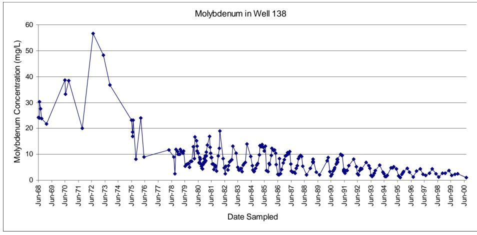
Figure 12. Molybdenum concentrations in Well 138
