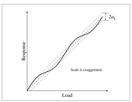
FIGURE 19.13 — Nonlinear balance response curve
