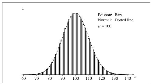
FIGURE 19.12b — Poisson distribution vs. normal distribution,  $\mu = 100$
