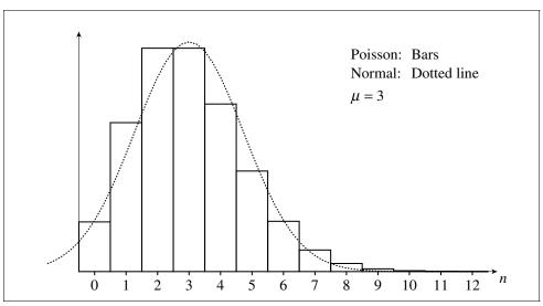
FIGURE 19.12a — Poisson distribution vs. normal distribution,  $\mu = 3$
