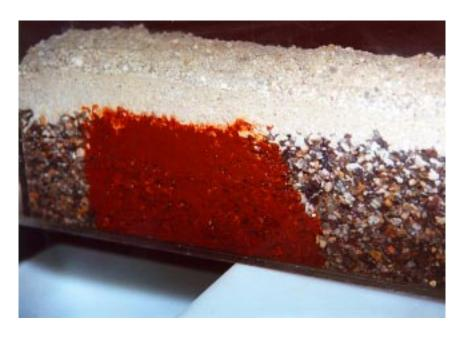
Figure 2.17. Testing hydraulic conductivity of amorphous ferric oxyhydroxide/gravel mixture.
