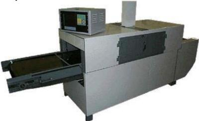
Figure D-2 Example Conveyorized Survey Monitoring System (Laurus 2001)
