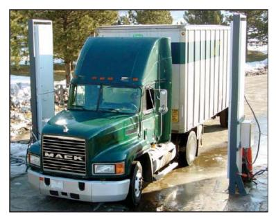
Figure D-3 Example Portal Monitor (Canberra 2005b)
