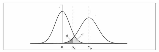
Figure 5.2 The Critical Value (S<sub>C</sub>) and the Minimum Detectable Value (S<sub>D</sub>) of the Net Instrument Signal (or Count)
