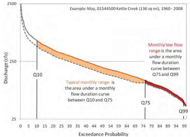
**Figure 17. Example flow duration curve that will be calculated from the modeled daily time series steps.**
