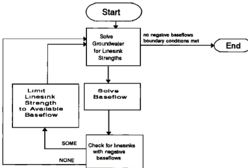
**Figure A30. Flowchart for coupling base flow and groundwater flow after Mitchell-Bruker (1996) as implemented in GFLOW.**
