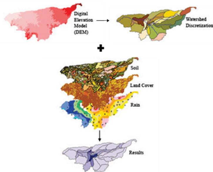
Figure A24. Schematic of data input layers used in SWAT and HSPF
