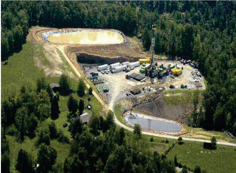
**Figure 5. Photograph of well pad with active hydraulic fracturing operations in the Marcellus shale. The upper reservoir is probably produced water.**
