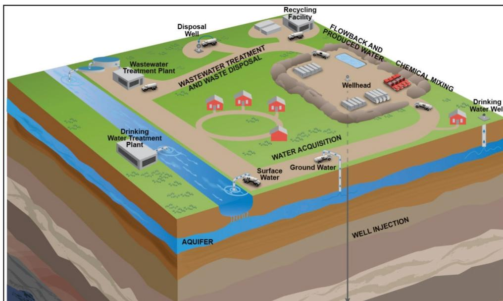
Figure 4. Sketch of typical hydraulic fracturing well pad.
