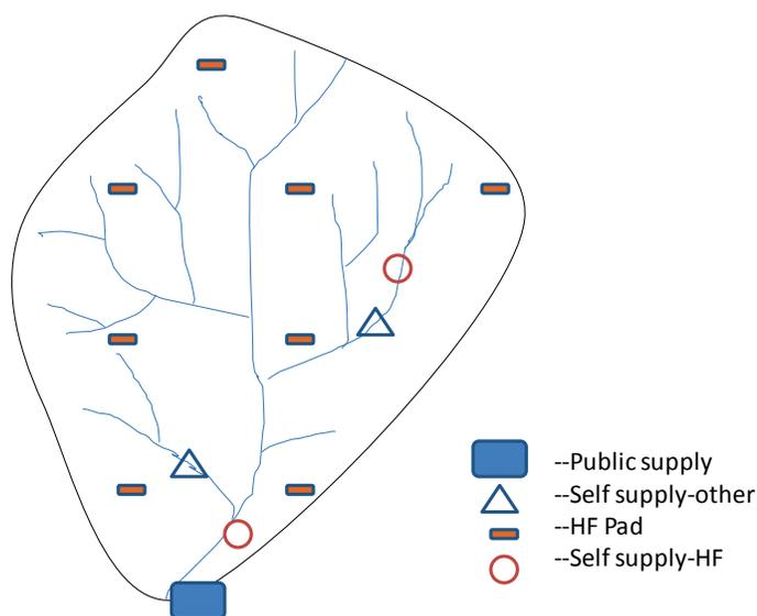
**Figure 19. Schematic of water withdrawal and hydraulic fracturing pads within subwatersheds.**
