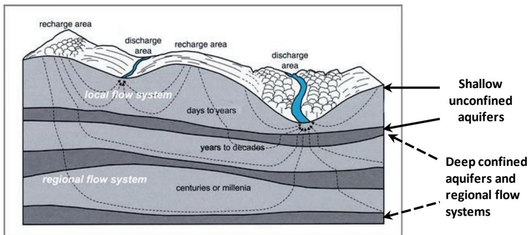
**Figure 13. Sketch of groundwater flow systems. (Graphic from U.S. Geological Survey).**
