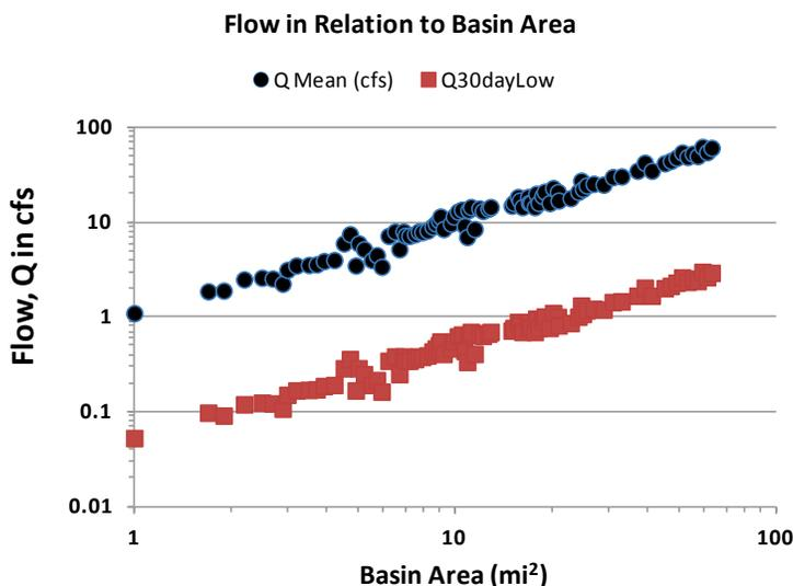
**Figure 18. Example relationship between discharge and basin area for two flow-duration statistics computed for Pennsylvania streams from a regional statistical analysis (Stuckey, 2006).**
