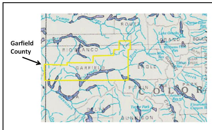
**Figure A6. The alluvial aquifers for Garfield County, Colorado (from Robson and Banta, 1995).**
