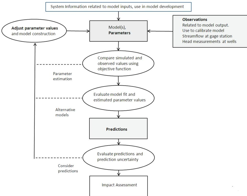
**Figure A31. The general ground water modeling workflow for this project will include the model parameterization phase and the model prediction phase with the objective to evaluate impact (after Hill and Tiedeman, 2007).**
