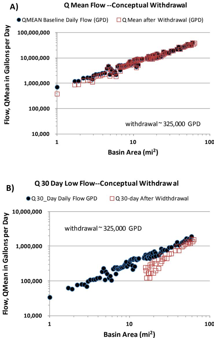
**Figure 20. Example calculation of withdrawal of 325,000 GPD on the annual mean flow and 30-day low flow of the Pennsylvania data set generated by the regional regression of discharge in relation to basin area (Stuckey, 2006).**
