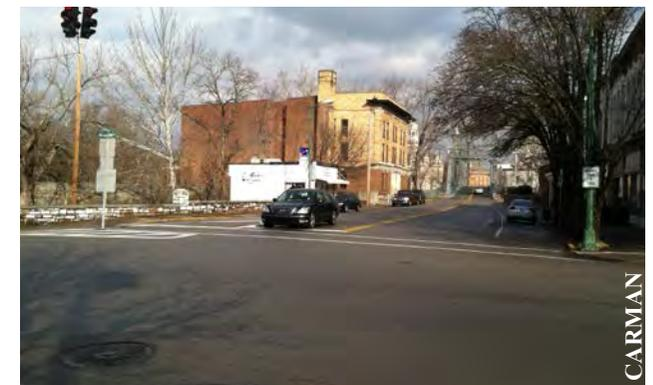
**Figure 14:** The crosswalk on Bridge Street at the intersection of Second Street is 70-feet long. Though there is a painted refuge in the middle of the crosswalk, it offers little safety for people crossing the road.
