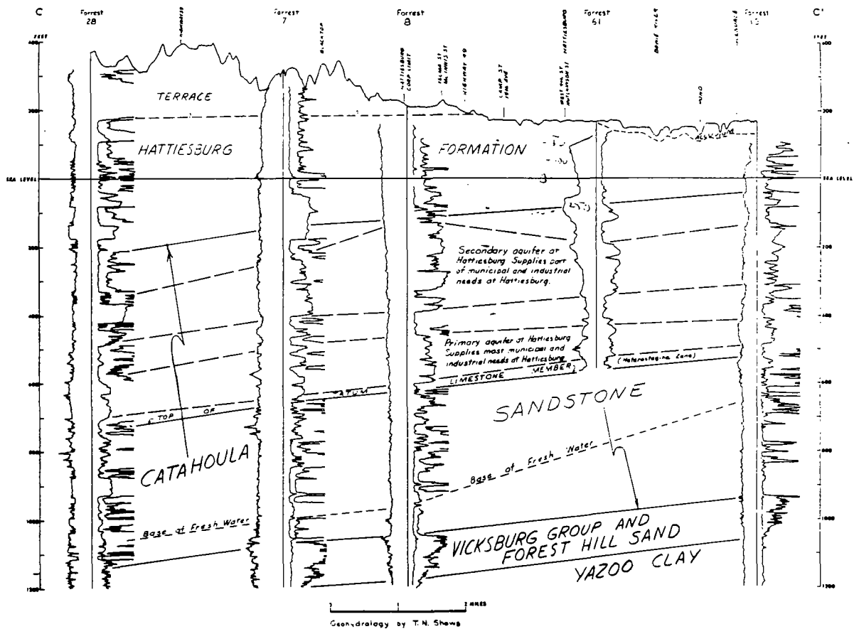
Fig. 22. Geohydrologic section (C-C') through the Hattiesburg area
