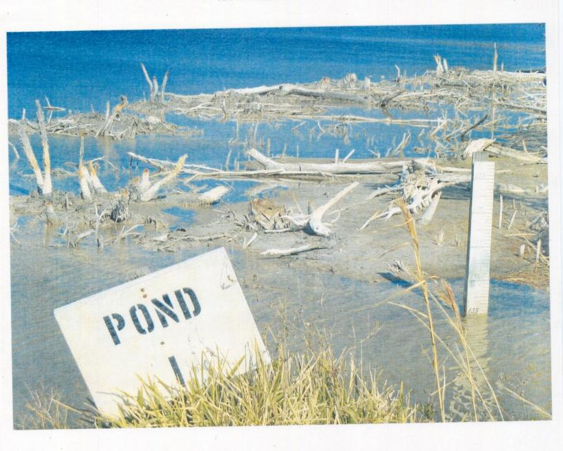
A staff gauge or a device for measuring water level in pond 1.
