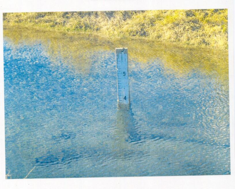
A staff gauge or a device for measuring water level in pond 4A.
