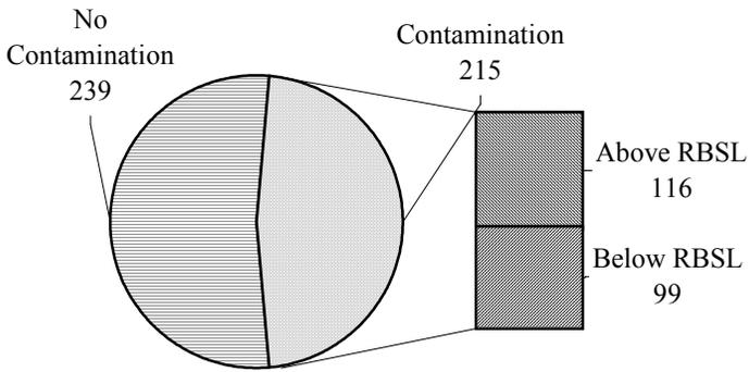
**Figure 2 - Contamination At 370 Facilities**
