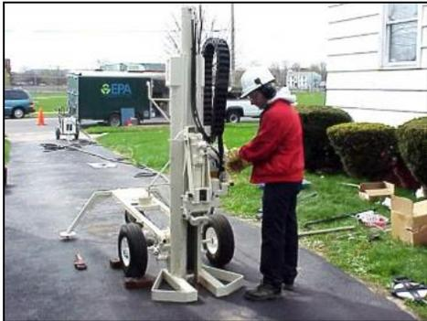
b) Percussion hammer system mounted on a track rig
