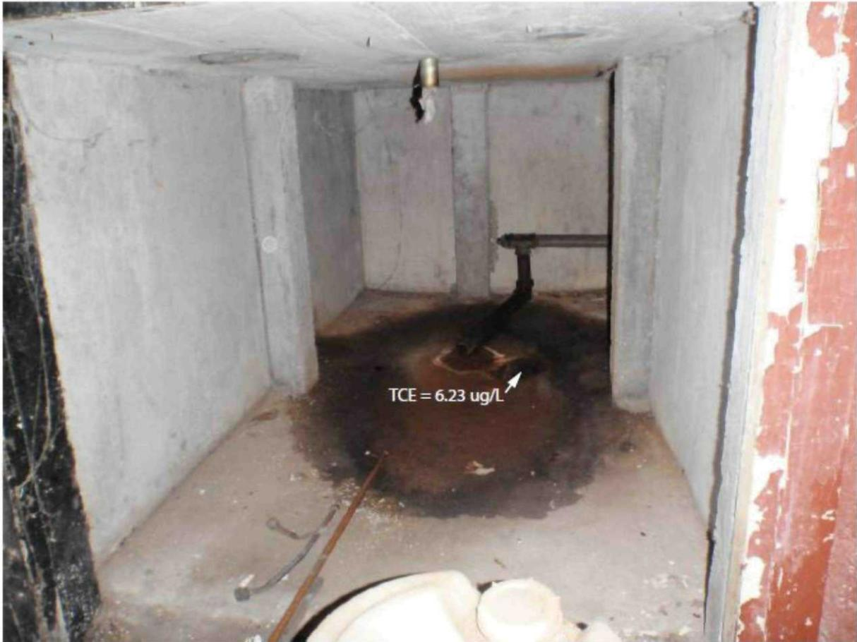
**Figure 4.** TCE concentration from a sampler placed in fluid-filled drain (arrow), former (alleged) Alabama Department of Transportation Laboratory.
