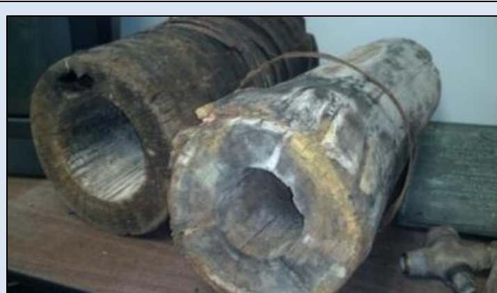
Exhibit B-1: Wooden and water and sewer pipes found in the Green Zone. Many of the water and sewer pipes in the Green Zone are over 80 years old. Despite the age of the system, city officials consider the system to be highly functional and safe.
