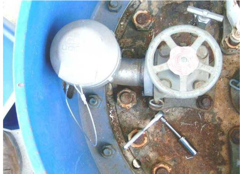
DryLok Fitting With Elbow Attached To Railcar Primary Valve
