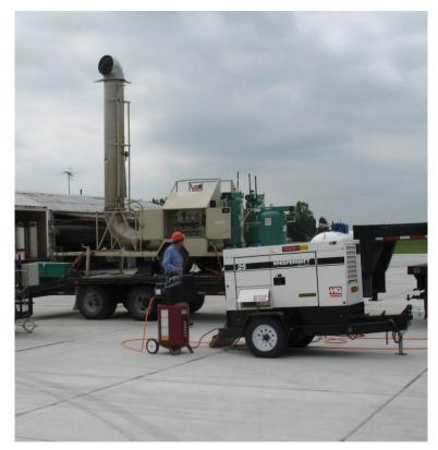
Figure 16. ASPECT Chemical Plume Generator. During this exercise, a controlled release of ammonia was used for the chemical agent.
