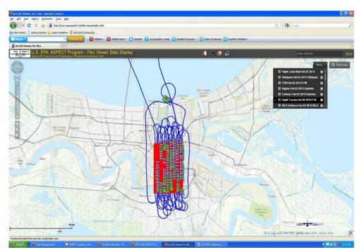
Figure 18. Sample ESRI Flex Viewer Display of ASPECT Aircraft Tracks. The red tracks indicate when radiological sensors were actively taking measurements.
