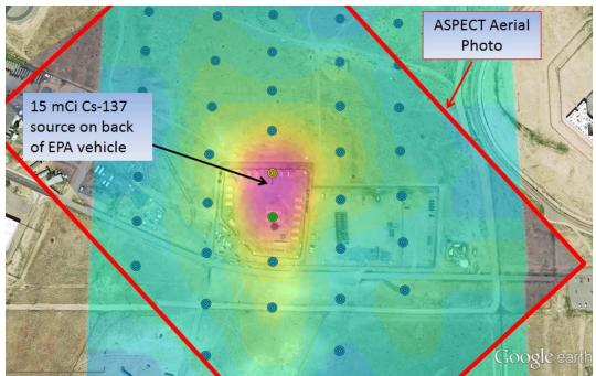
Figure 13. Cs-137 region-of-interest count-rate contour overlaid on the sigma plot. This product can be produced within minutes and can be used to plan a ground-based survey.
