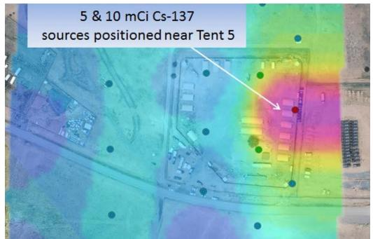
Figure 14. Cs-137 region-of-interest count-rate contour overlaid on the sigma plot after the sources were moved to the new location.
