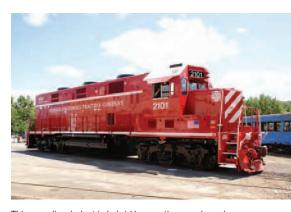
This new diesel-electric hybrid locomotive, purchased with partial funding from EPA, is cleaner and uses 50% less fuel than its predecessor on a freight line in California's San Joaquin Valley. Far right: Improved air quality in Los Angeles.
