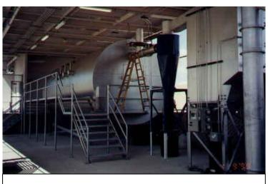
Figure 2. Semi-continuous system uses solid fuel as ignition source for wastes
