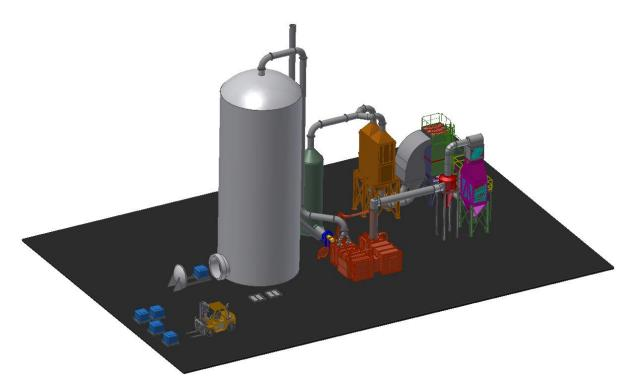
Figure 10. Minden Contained Burn System Layout, with All PAS Options Shown
