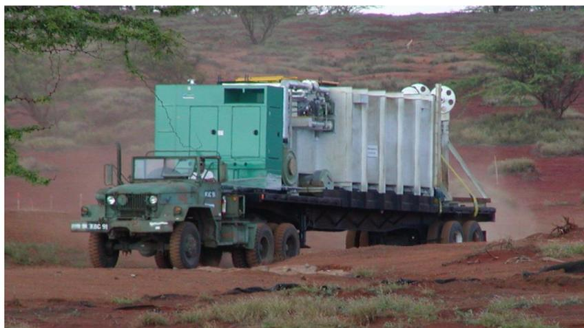
**Figure 3: Transportable Flashing Furnace**
