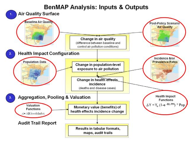
Figure 1-3. BenMAP-CE Flow Diagram
