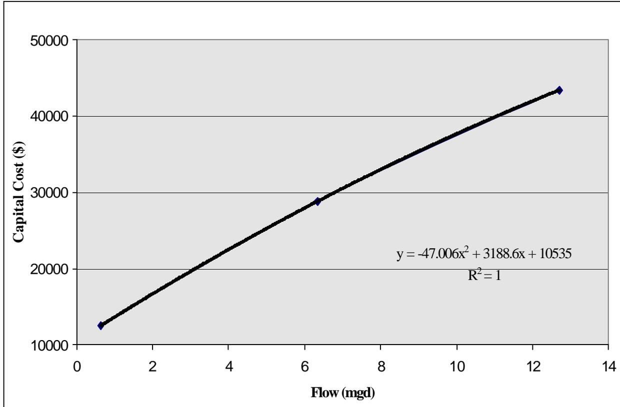
**Figure 3-50. O&M Costs for Enlarging Intake Externally with Stainless Steel Fine Mesh Screen**
