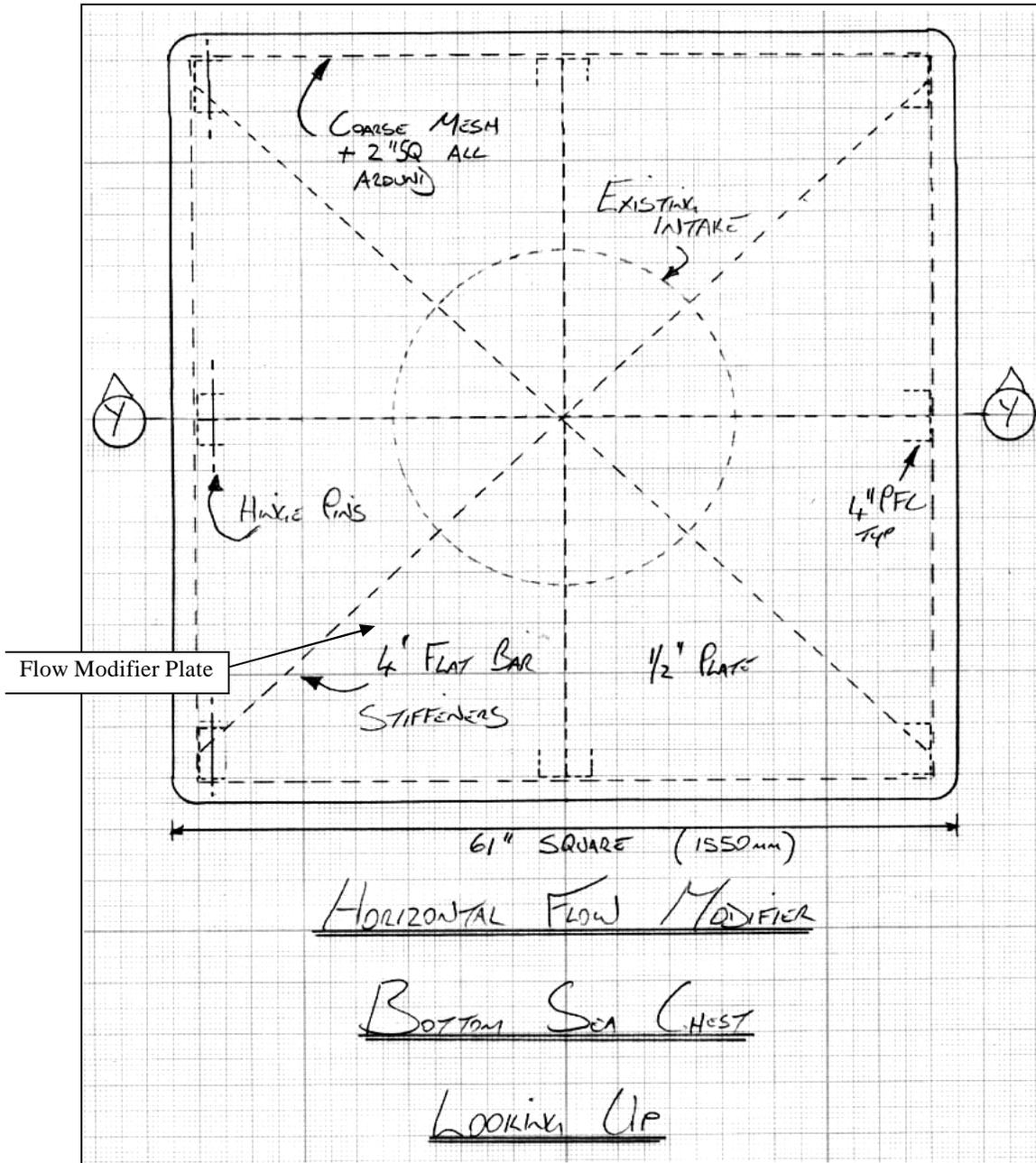
Figure 3-54. Sectional View of Bottom Sea Chest Horizontal Flow Modifier
