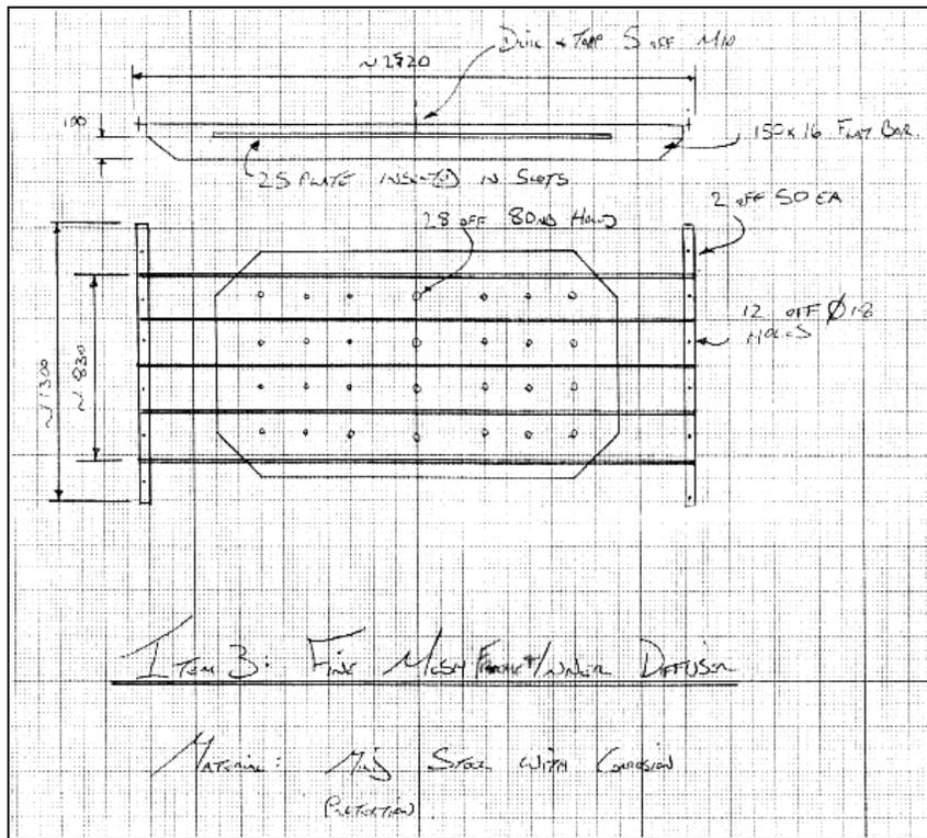
**Figure 3-42. Main Frame for Internal Intake Modification**
