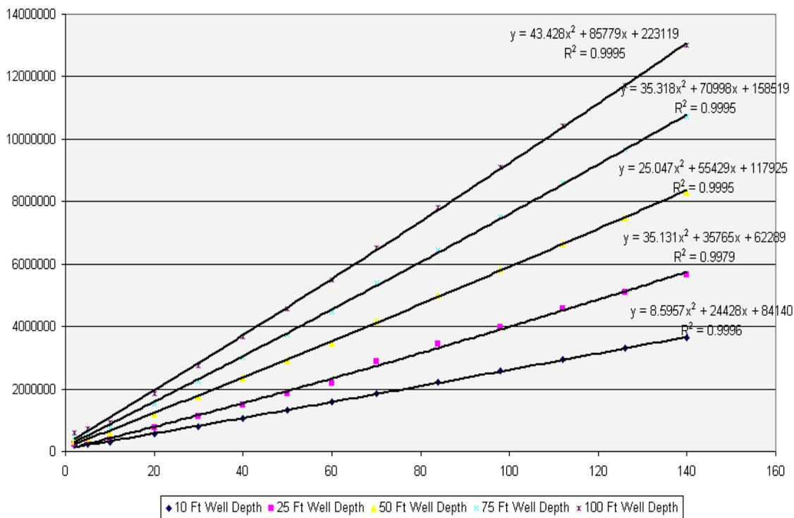
**Figure 3-23. Scenario C – Capital Cost – Add Fine Mesh Traveling Screen with Fish Handling and Return - Freshwater**
