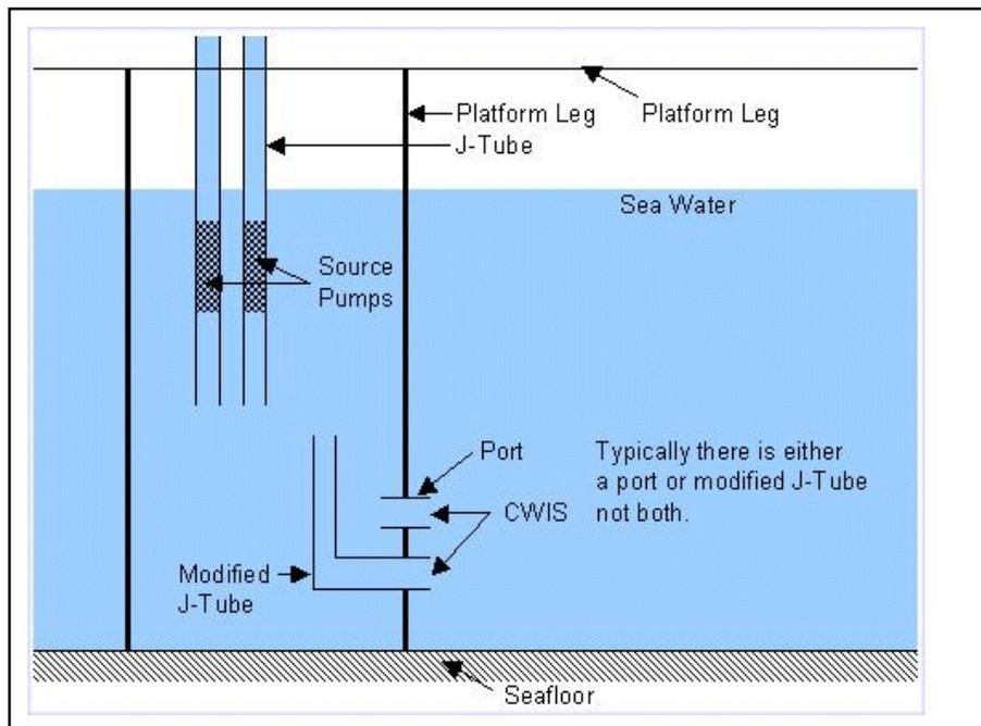
Note: Another configuration, the “J” Tube configuration, also uses simple pipes as a cooling water intake structure but with no seawater in the platform leg.
