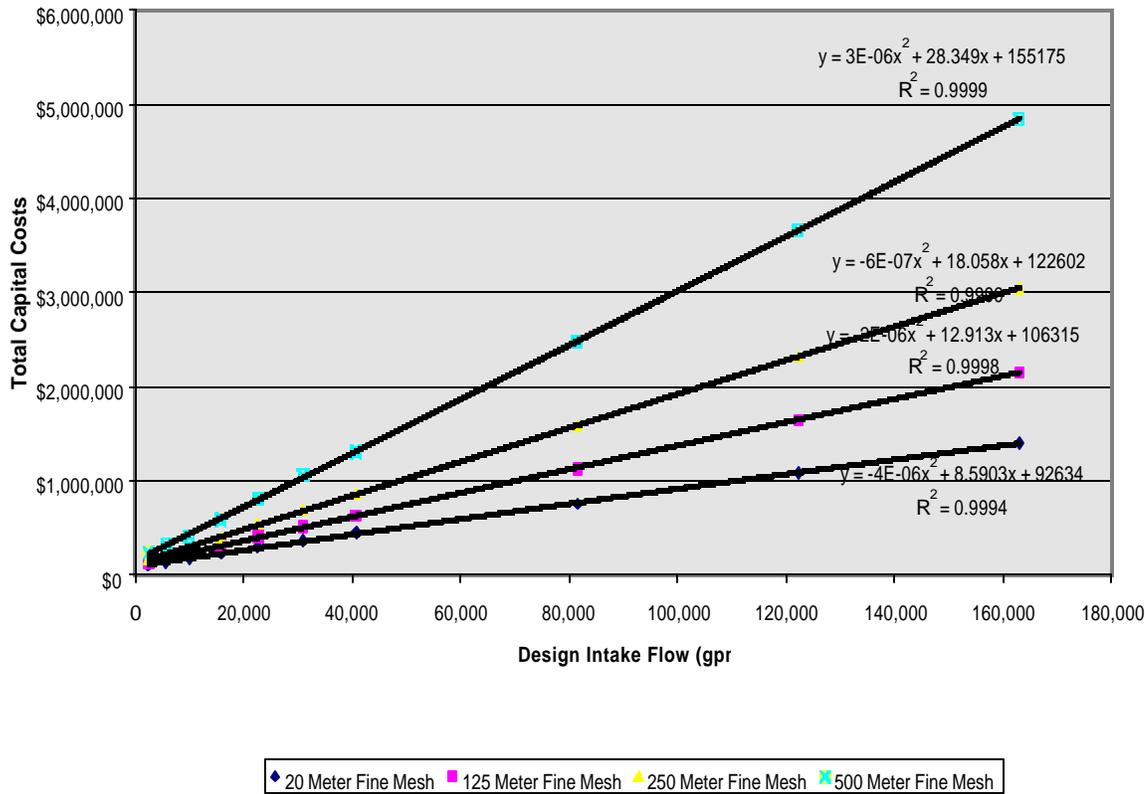
**Figure 3-13. Capital Costs for Very Fine Mesh Passive Screen Existing Offshore in Freshwater at Selected Offshore Distances**
