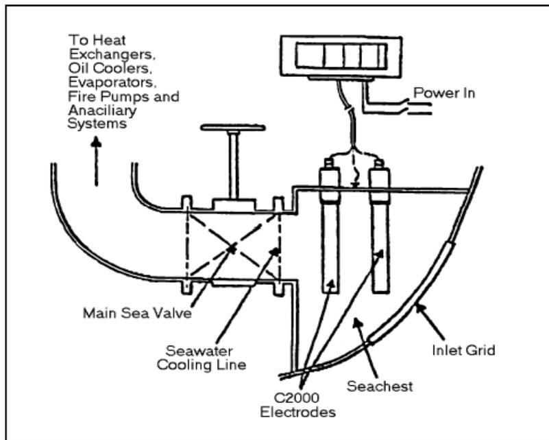
Figure 7-3. Offshore Simple Pipe Cooling Water Intake Structure Design (Schematic)
