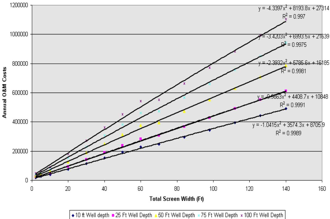
**Figure 3-27. Scenarios A&C Compliance O&M Total Costs for Traveling Screens with Fish Handling – Saltwater Environments**
