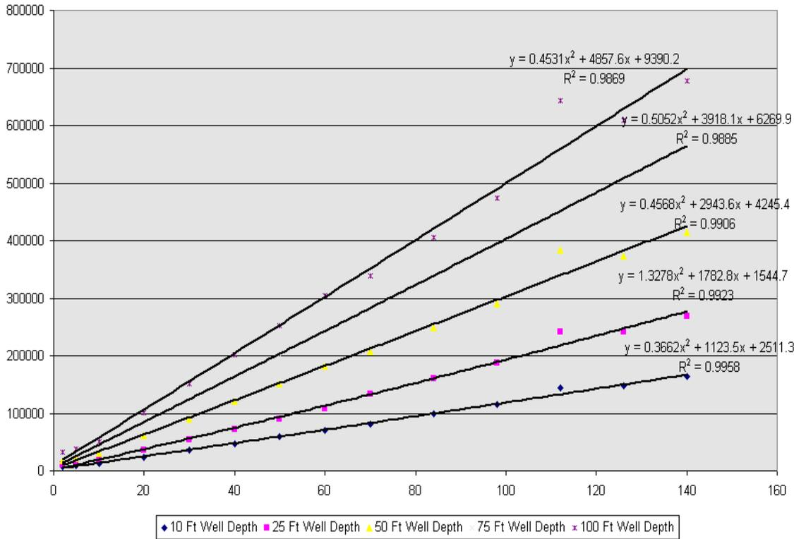
**Figure 3-19. Scenario A – Capital Cost – Add Fine Mesh Replacement Screen Panels - Saltwater**
