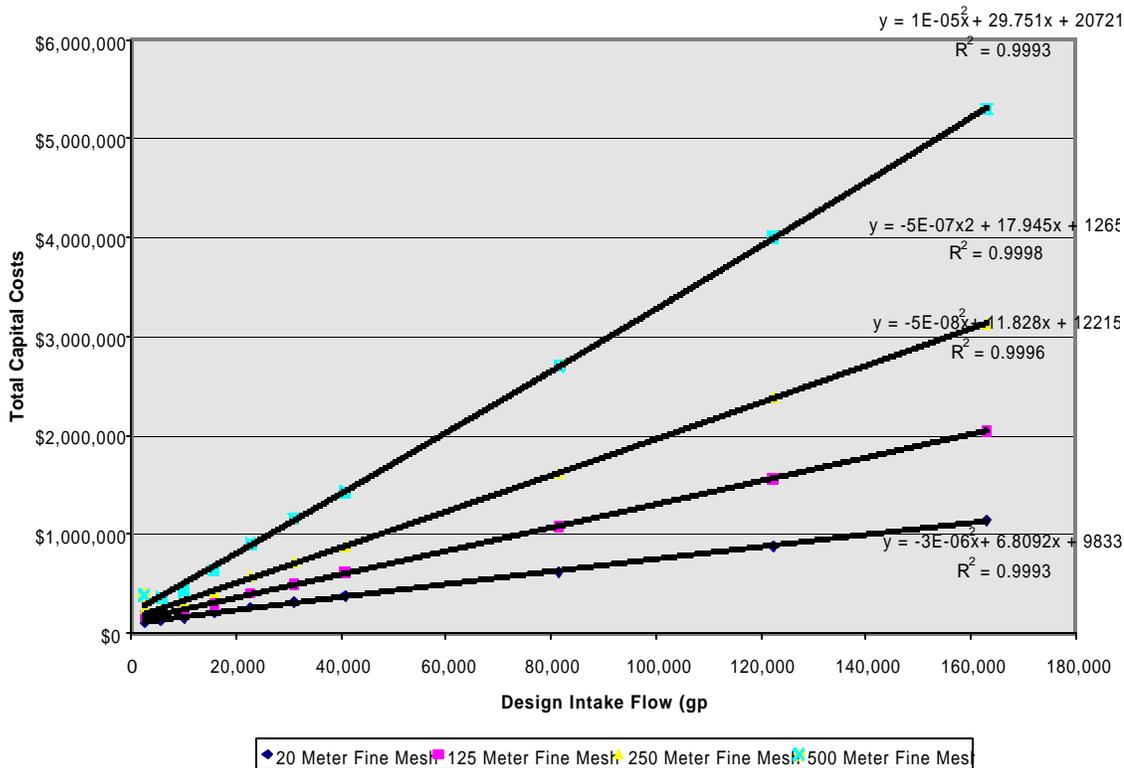
**Figure 3-12. Capital Costs for Fine Mesh Passive Screen Existing Offshore in Freshwater with Zebra Mussels at Selected Offshore Distances**
