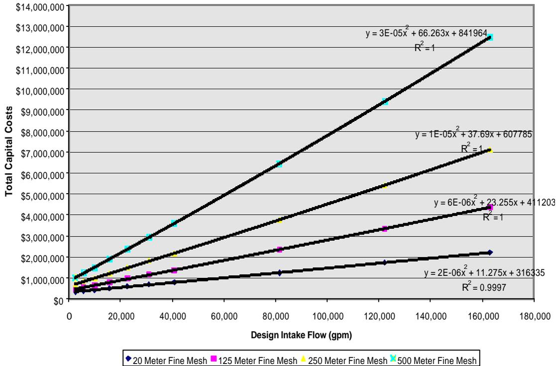
**Exhibit 3-11. Total Capital Costs of Installed Very Fine Mesh T-screen System at Existing Shoreline Based Intakes**
