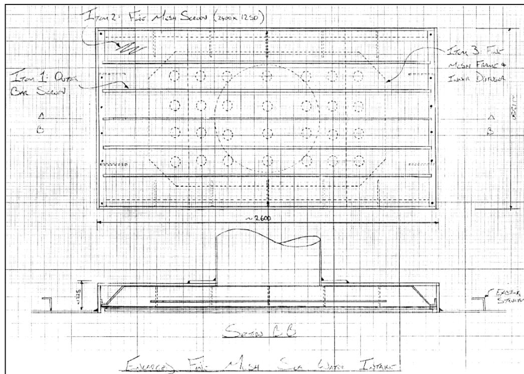
**Figure 3-39. Outer Bar Screen (for Internal and External Intake Modification)**
