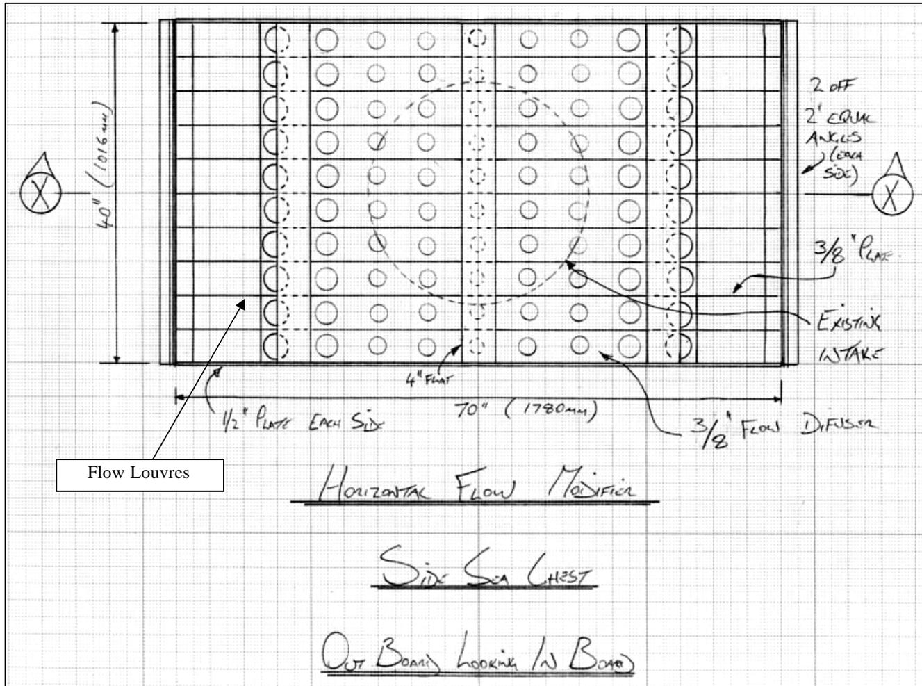
**Figure 3-56. Sectional View of Side Sea Chest Horizontal Flow Modifier**
