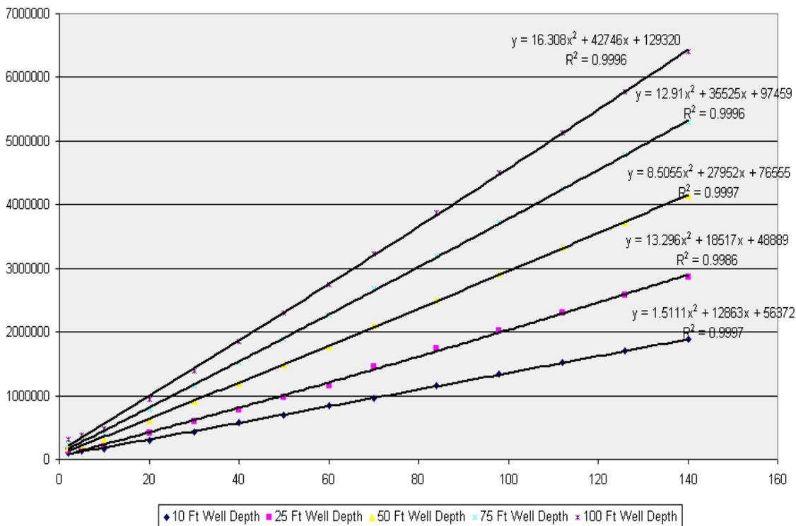
**Figure 3-21. Scenario B – Capital Cost – Add Traveling Screen with Fish Handling and Return - Saltwater**
