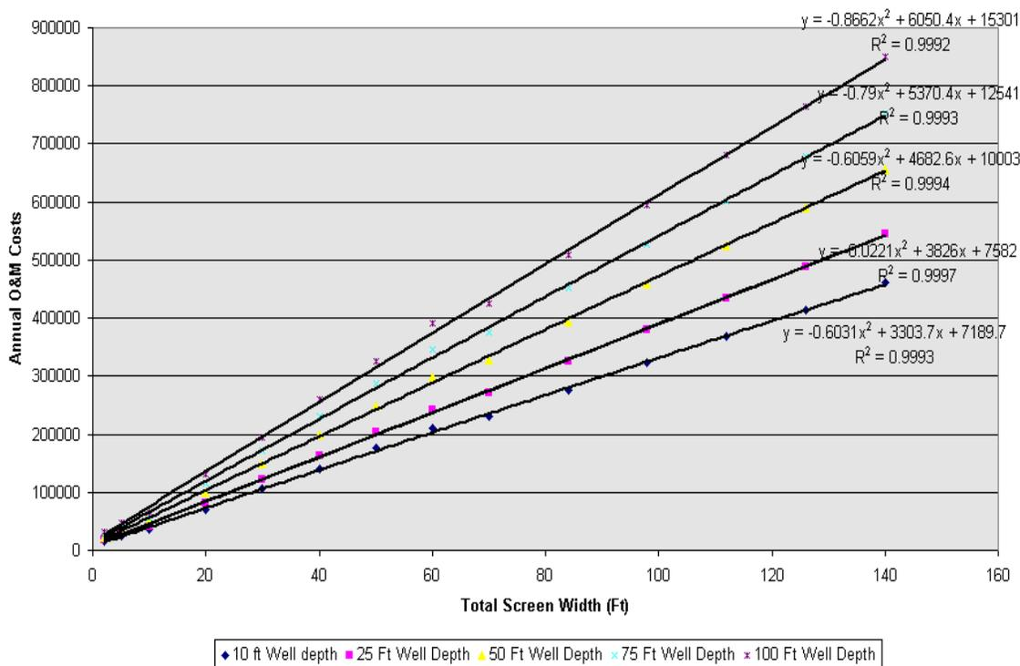
**Figure 3-29. Baseline & Scenarios B Compliance O&M Total Costs for Traveling Screens with Fish Handling - Saltwater Environments**
