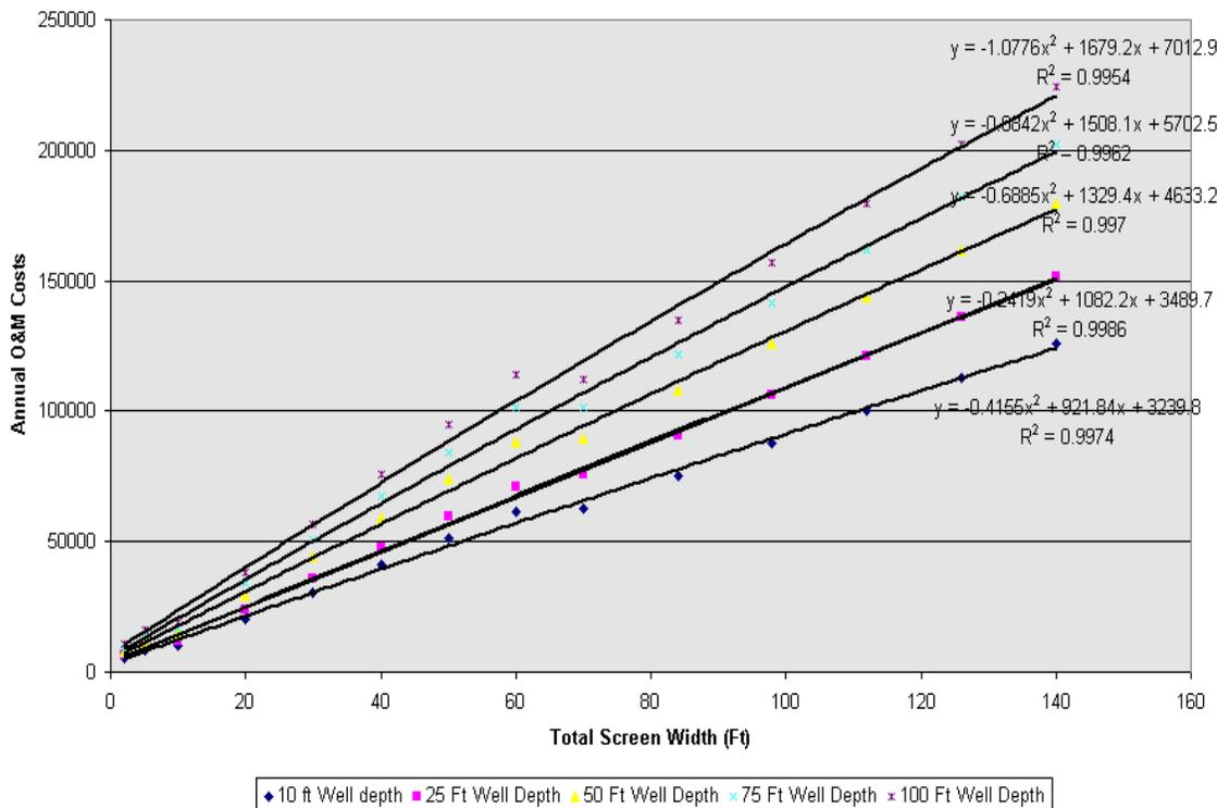
**Figure 3-25. Baseline O&M Costs for Traveling Screens without Fish Handling – Saltwater Environments**
