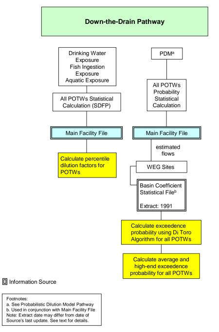
Figure 3-1 Exposure and Fate Assessment Screening Tool, Version 2.0 (E-FAST2) Down-the-Drain Pathway (Surface Water Discharge Information Organization and Sources)
