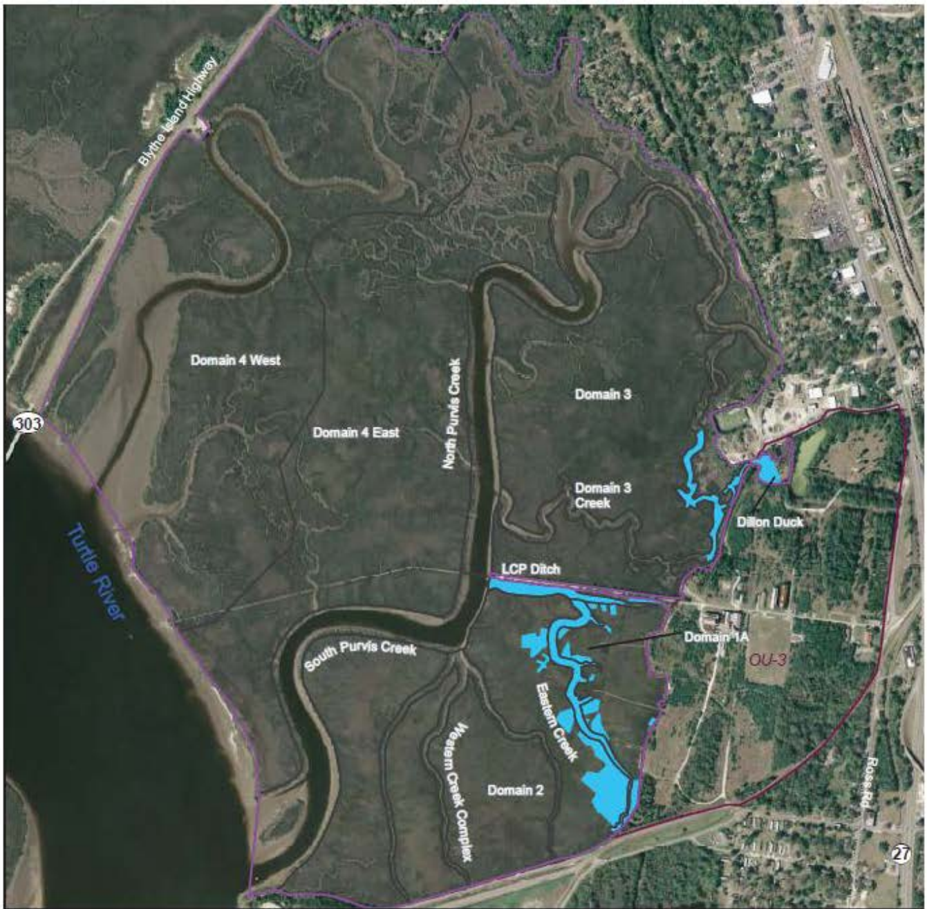
Figure 9 – Sediment Remedy Alternative 4: Sediment Removal – 18 Acres
