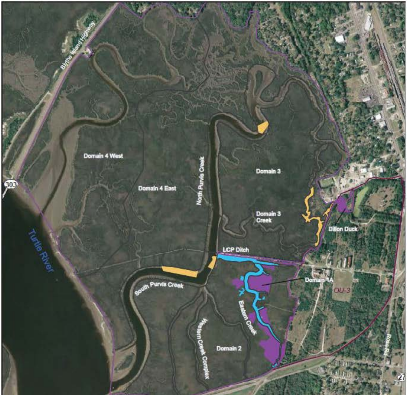
Figure 11 – Sediment Remedy Alternative 6: Sediment Removal, Capping, and Thin Cover – 24 Acres
