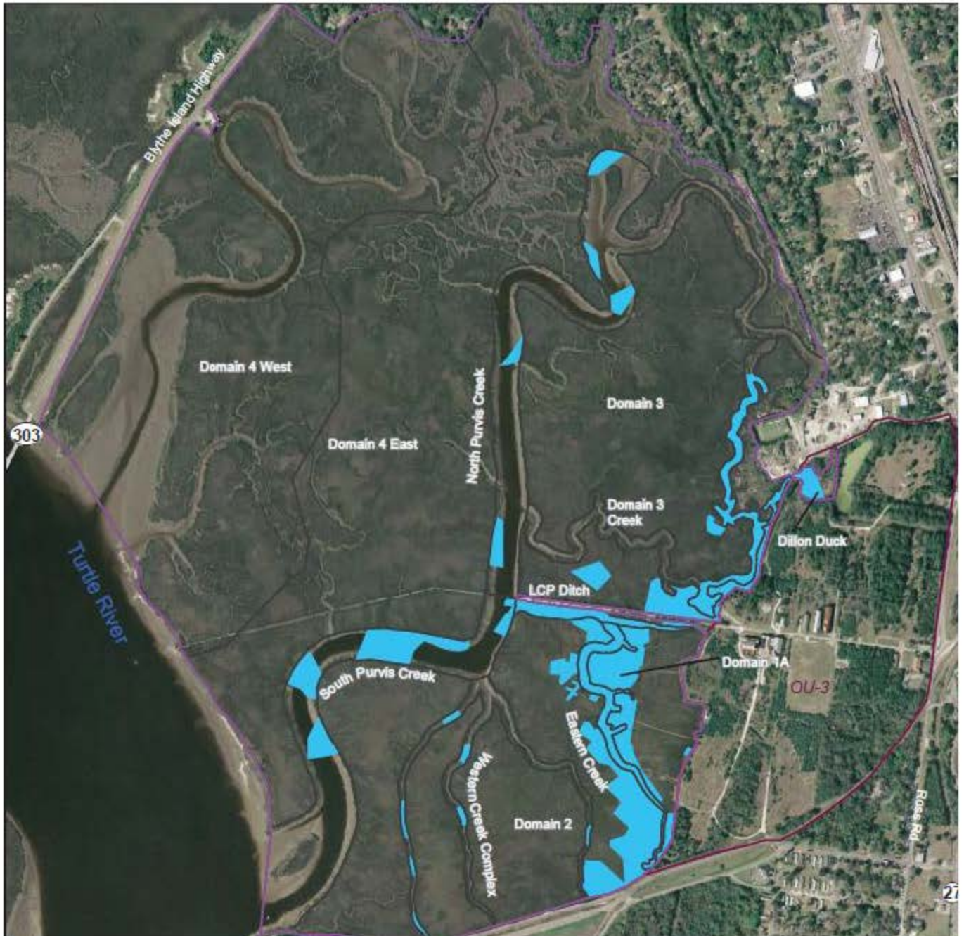
Figure 7 – Sediment Remedy Alternative 2: Sediment Removal – 48 Acres
