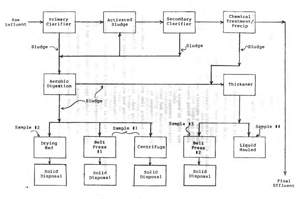
Figure 1. POTW "Generic" Flow Diagram
