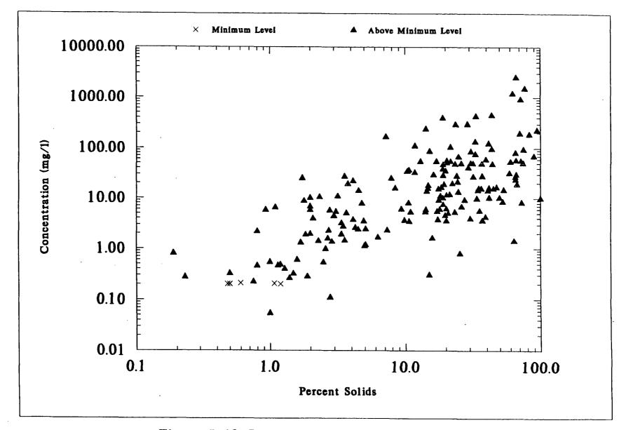
Figure 7-18. Percent Solids of NSSS Samples Versus WET WEIGHT Concentrations of CHROMIUM
