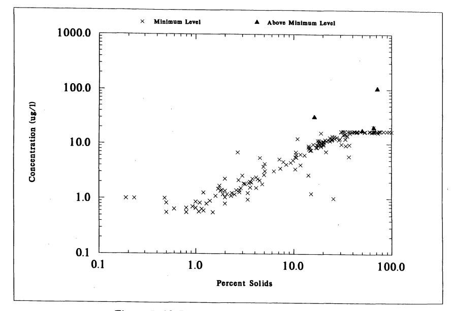
Figure 7-66. Percent Solids of NSSS Samples Versus WET WEIGHT Concentrations of 4.4-DDE
