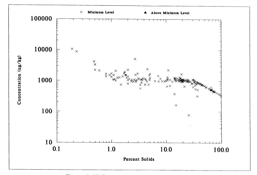
Figure 7-57. Percent Solids of NSSS Samples Versus DRY WEIGHT Concentrations of TOXAPHENE
