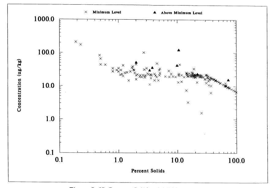
Figure 7-67. Percent Solids of NSSS Samples Versus DRY WEIGHT Concentrations of 4.4 - DDT
