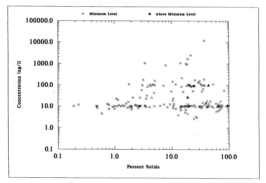
Figure 7-6. Percent Solids of NSSS Samples Versus WET WEIGHT Concentrations of BENZENE
