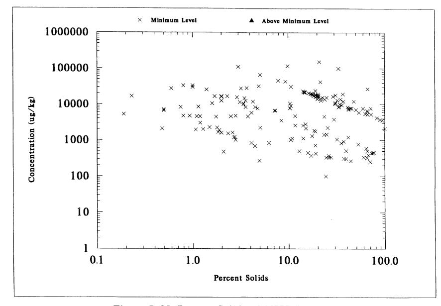
Figure 7-25. Percent Solids of NSSS Samples Versus DRY WEIGHT Concentrations of HEXACHLOROBENZENE
