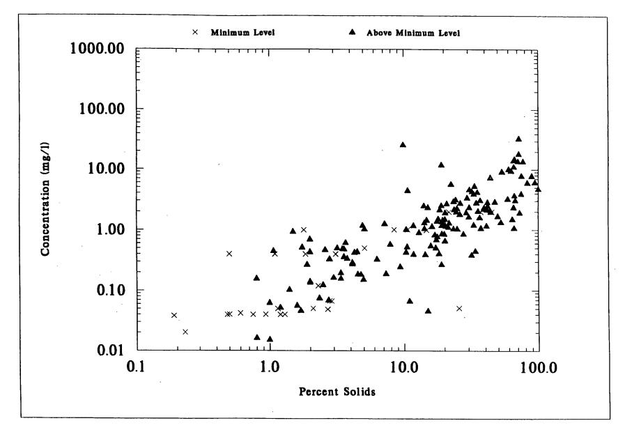
Figure 7-4. Percent Solids of NSSS Samples Versus WET WEIGHT Concentrations of ARSENIC
