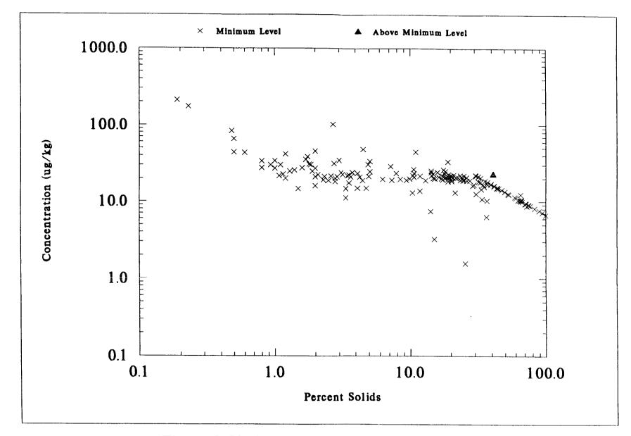
Figure 7-23. Percent Solids of NSSS Samples Versus DRY WEIGHT Concentrations of HEPTACHLOR
