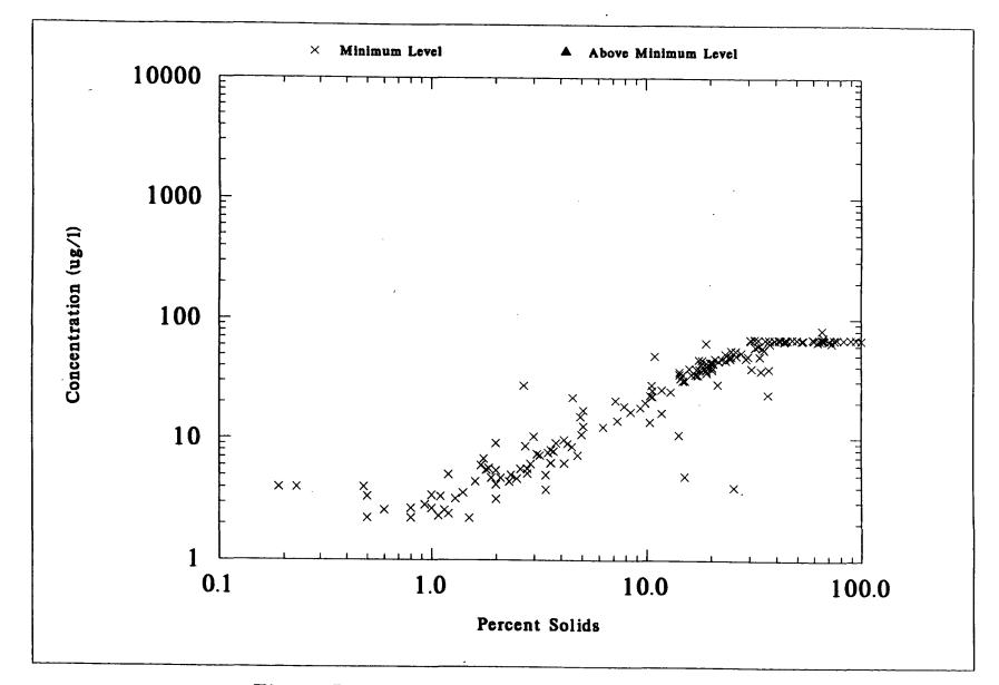
Figure 7-44. Percent Solids of NSSS Samples Versus WET WEIGHT Concentrations of PCB-1221
