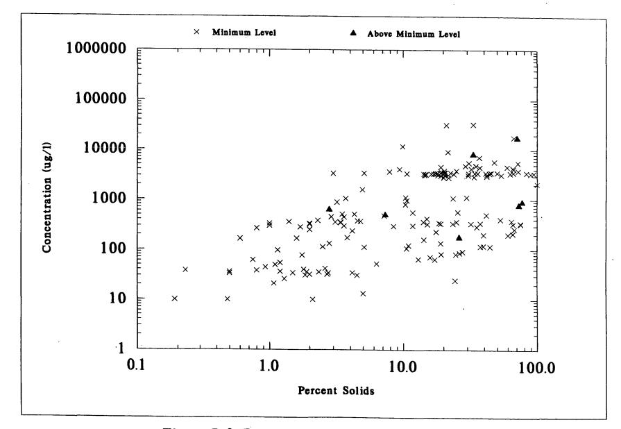
Figure 7-8. Percent Solids of NSSS Samples Versus WET WEIGHT Concentrations of BENZO(A)PYRENE
