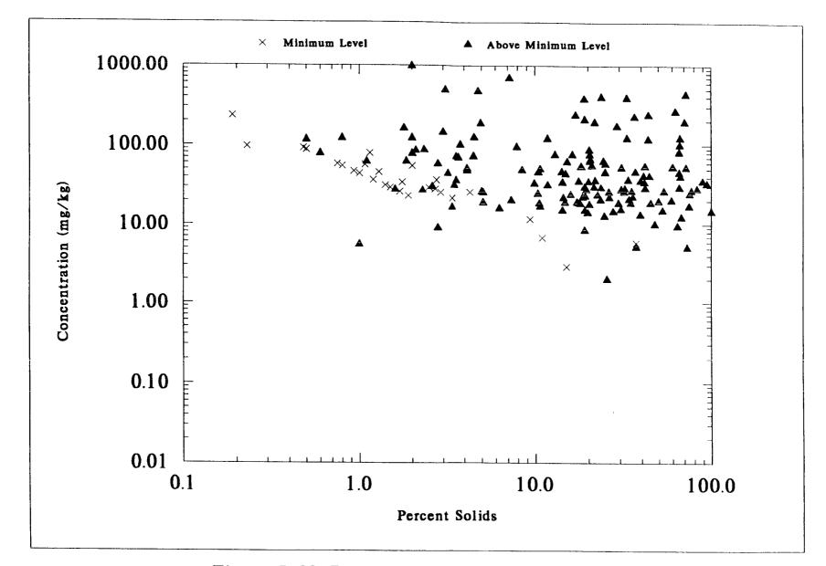
Figure 7-39. Percent Solids of NSSS Samples Versus DRY WEIGHT Concentrations of NICKEL
