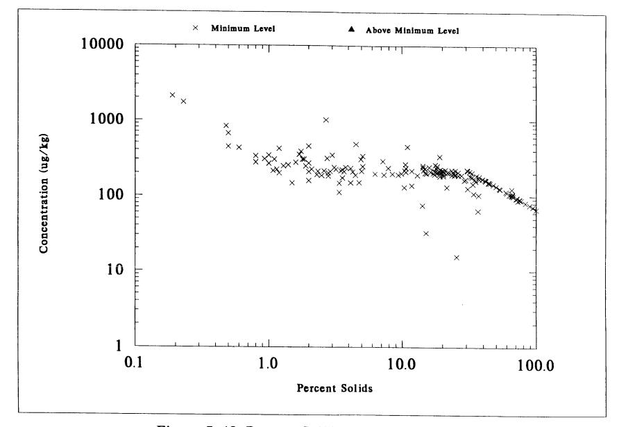
Figure 7-45. Percent Solids of NSSS Samples Versus DRY WEIGHT Concentrations of PCB-1232
