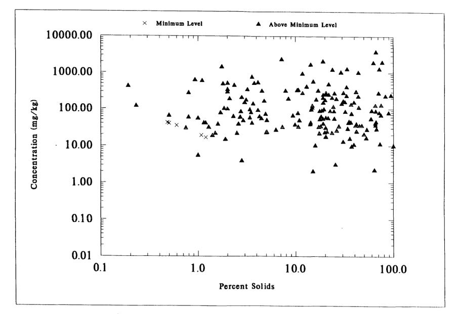
Figure 7-17. Percent Solids of NSSS Samples Versus DRY WEIGHT Concentrations of CHROMIUM
