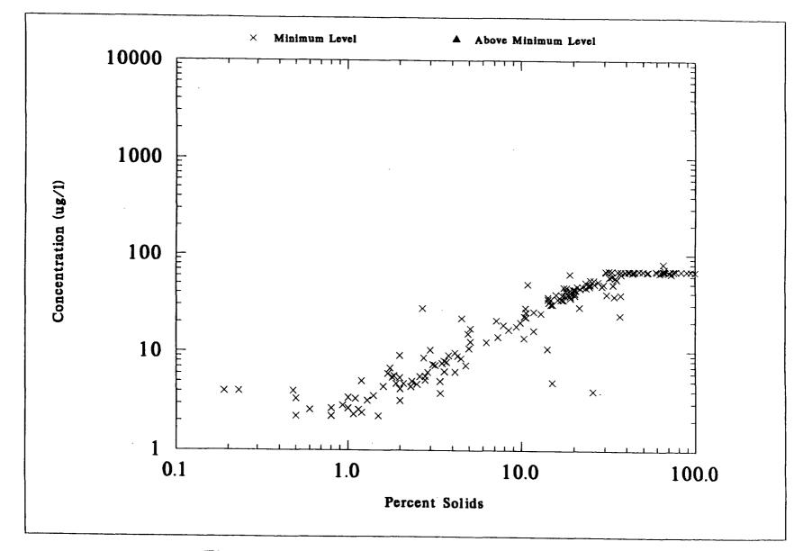
Figure 7-48. Percent Solids of NSSS Samples Versus WET WEIGHT Concentrations of PCB-1242
