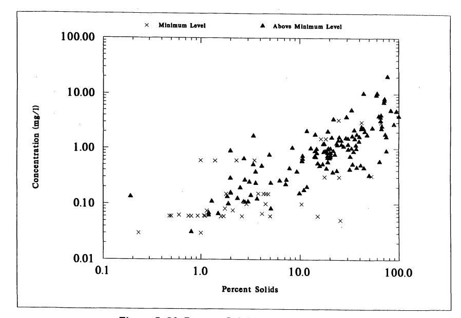
Figure 7-56. Percent Solids of NSSS Samples Versus WET WEIGHT Concentrations of SELENIUM
