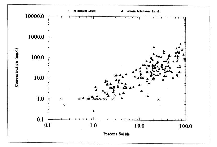
Figure 7-30. Percent Solids of NSSS Samples Versus WET WEIGHT Concentrations of LEAD
