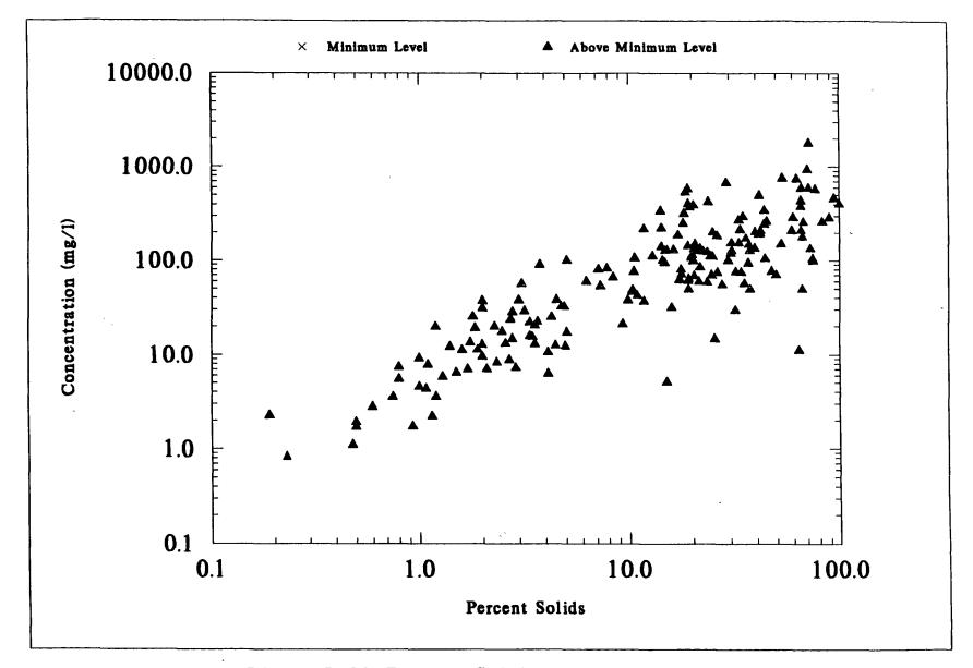
Figure 7-20. Percent Solids of NSSS Samples Versus WET WEIGHT Concentrations of COPPER
