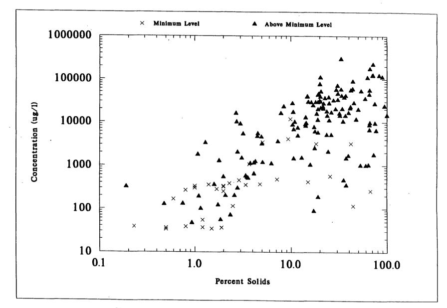
Figure 7-12. Percent Solids of NSSS Samples Versus WET WEIGHT Concentrations of BIS(2-ETHYLHEXYL) PHTHALATE
