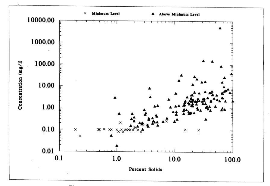
Figure 7-14. Percent Solids of NSSS Samples Versus WET WEIGHT Concentrations of CADMIUM
