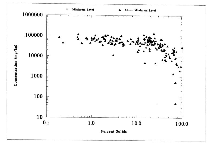
Figure 7-71. Percent Solids of NSSS Samples Versus DRY WEIGHT Concentrations of TOTAL KJELDAHL NITROGEN
