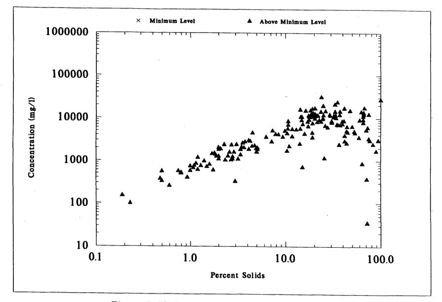
Figure 7-72. Percent Solids of NSSS Samples Versus WET WEIGHT Concentrations of TOTAL KJELDAHL NITROGEN
