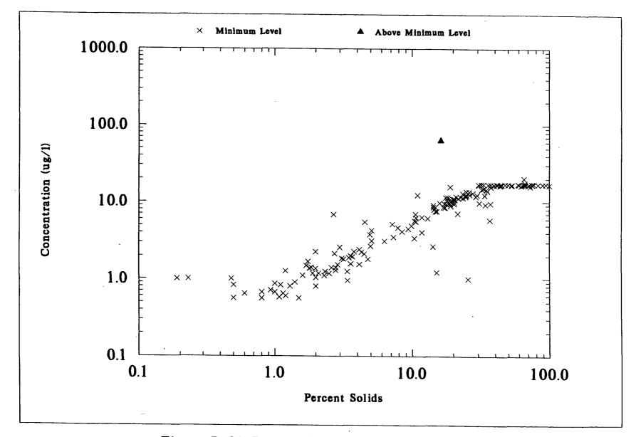
Figure 7-64. Percent Solids of NSSS Samples Versus WET WEIGHT Concentrations of 4.4-DDD
