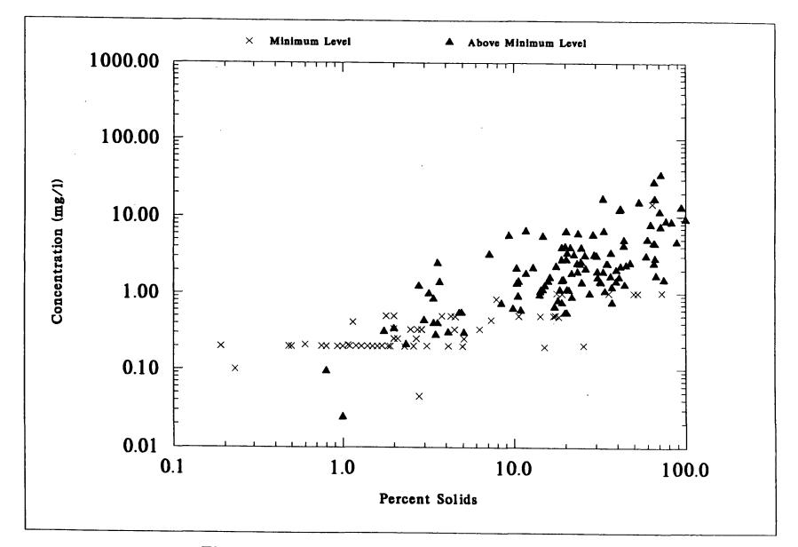
Figure 7-36. Percent Solids of NSSS Samples Versus WET WEIGHT Concentrations of MOLYBDENUM
