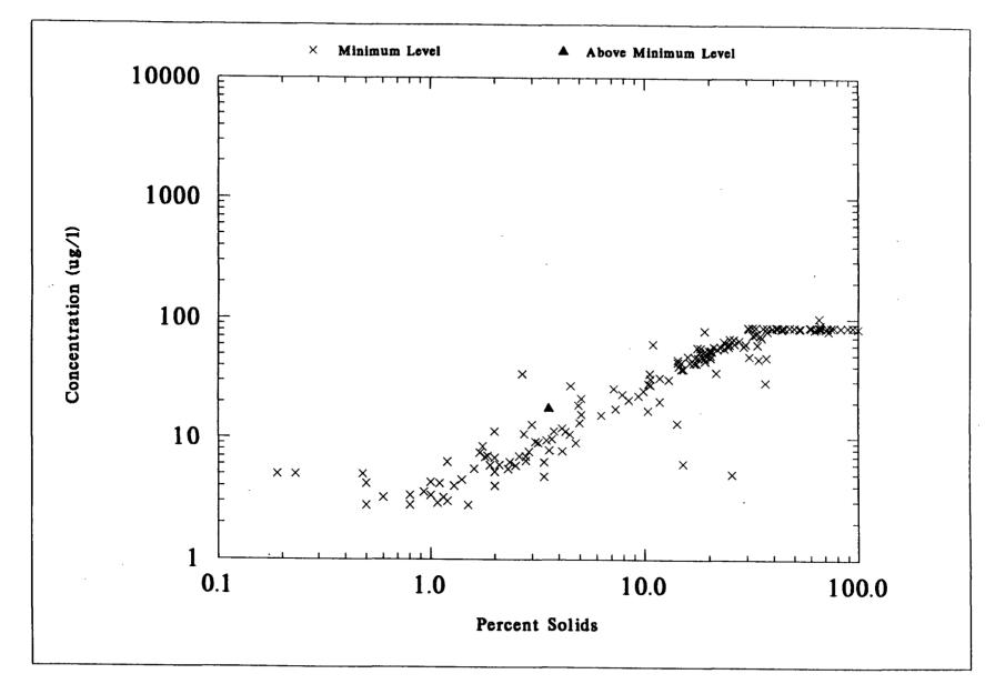
Figure 7-16. Percent Solids of NSSS Samples Versus WET WEIGHT Concentrations of CHLORDANE
