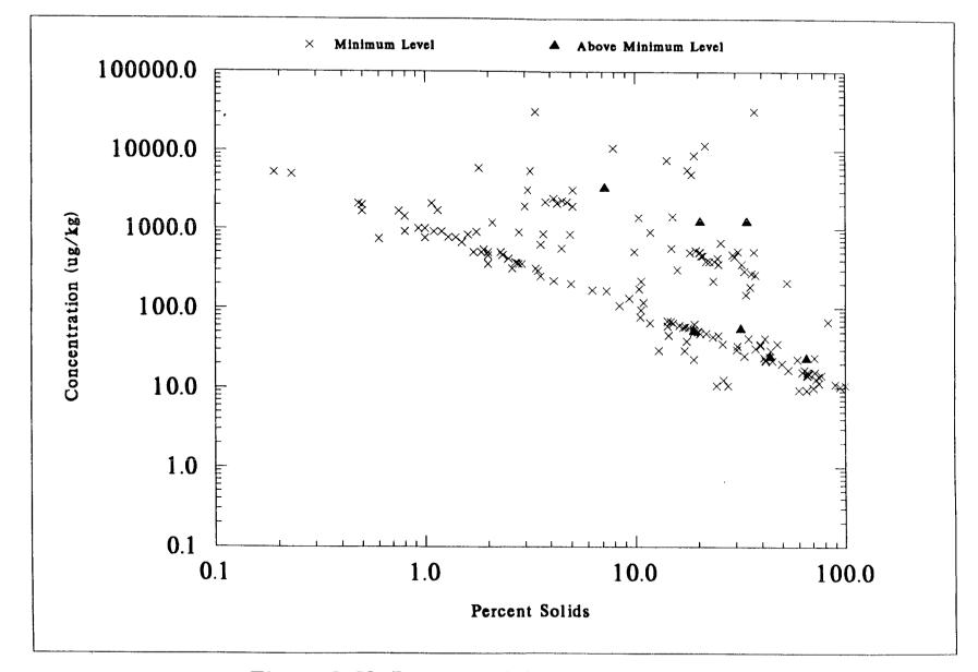
Figure 7-59. Percent Solids of NSSS Samples Versus DRY WEIGHT Concentrations of TRICHLOROETHENE
