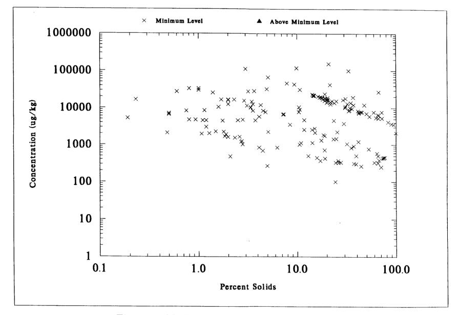
Figure 7-27. Percent Solids of NSSS Samples Versus DRY WEIGHT Concentrations of HEXACHLOROBUTADIENE
