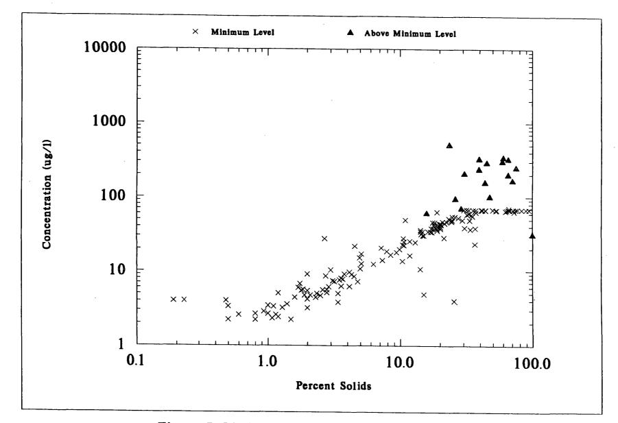
Figure 7-54. Percent Solids of NSSS Samples Versus WET WEIGHT Concentrations of PCB-1260
