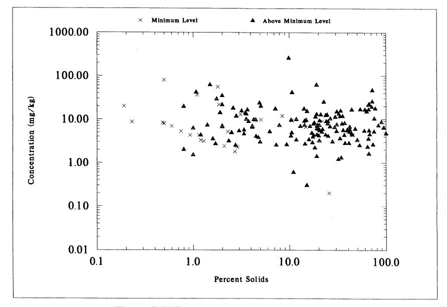
Figure 7-3. Percent Solids of NSSS Samples Versus DRY WEIGHT Concentrations of ARSENIC
