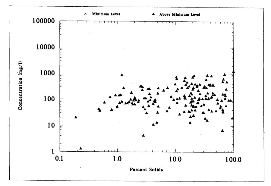
Figure 7-70. Percent Solids of NSSS Samples Versus WET WEIGHT Concentrations of PHOSPHORUS
