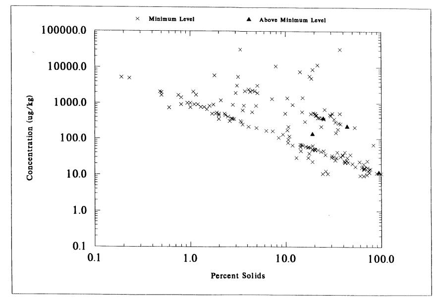
Figure 7-5. Percent Solids of NSSS Samples Versus DRY WEIGHT Concentrations of BENZENE
