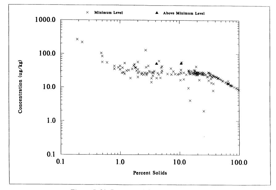
Figure 7-31. Percent Solids of NSSS Samples Versus DRY WEIGHT Concentrations of LINDANE (GAMMA-BHC)
