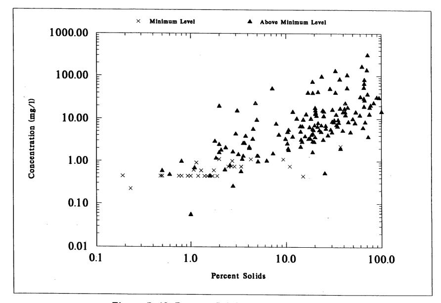
Figure 7-40. Percent Solids of NSSS Samples Versus WET WEIGHT Concentrations of NICKEL
