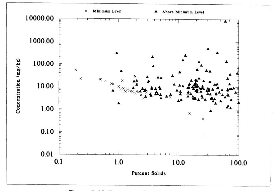
Figure 7-13. Percent Solids of NSSS Samples Versus DRY WEIGHT Concentrations of CADMIUM
