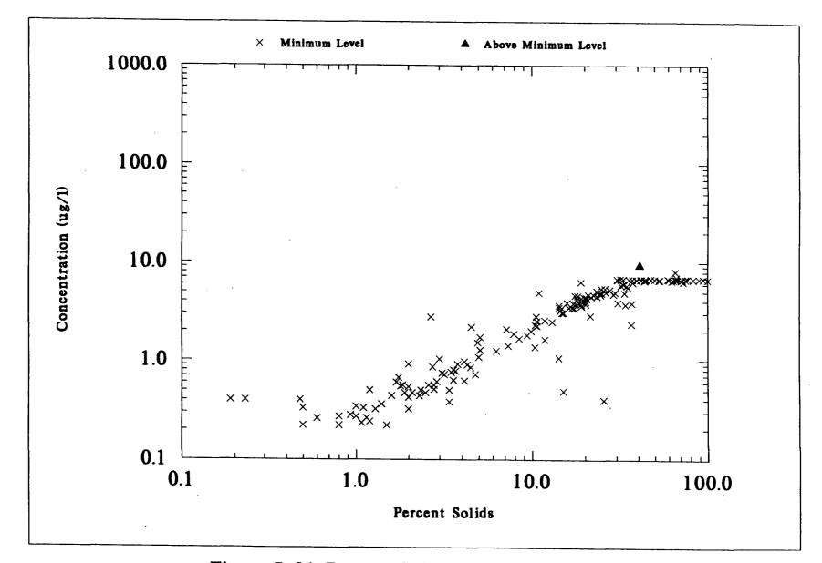
Figure 7-24. Percent Solids of NSSS Samples Versus WET WEIGHT Concentrations of HEPTACHLOR
