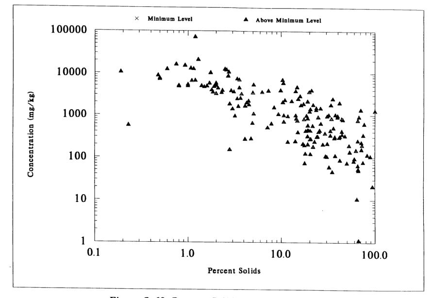
Figure 7-69. Percent Solids of NSSS Samples Versus DRY WEIGHT Concentrations of PHOSPHORUS
