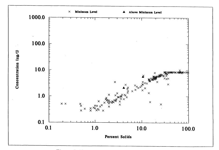
Figure 7-32. Percent Solids of NSSS Samples Versus WET WEIGHT Concentrations of LINDANE (GAMMA-BHC)
