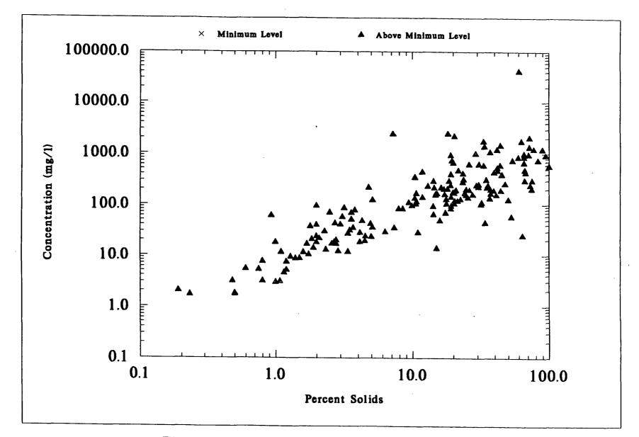
Figure 7-62. Percent Solids of NSSS Samples Versus WET WEIGHT Concentrations of ZINC
