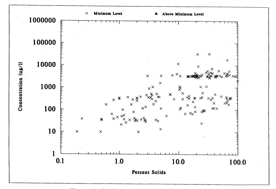
Figure 7-28. Percent Solids of NSSS Samples Versus WET WEIGHT Concentrations of HEXACHLOROBUTADIENE
