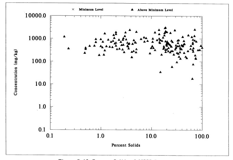
Figure 7-19. Percent Solids of NSSS Samples Versus DRY WEIGHT Concentrations of COPPER
