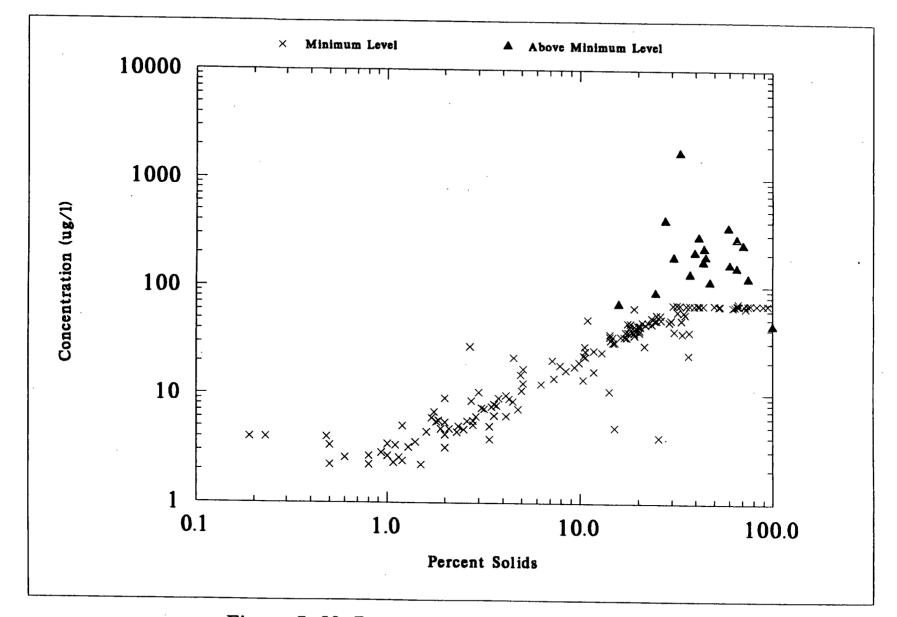
Figure 7-50. Percent Solids of NSSS Samples Versus WET WEIGHT Concentrations of PCB-1248
