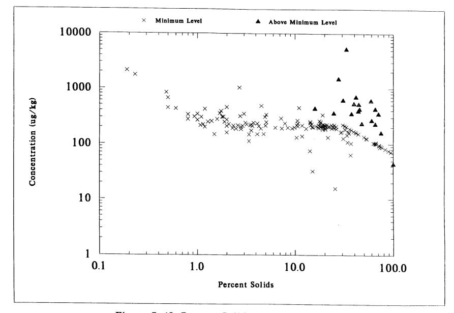
Figure 7-49. Percent Solids of NSSS Samples Versus DRY WEIGHT Concentrations of PCB-1248
