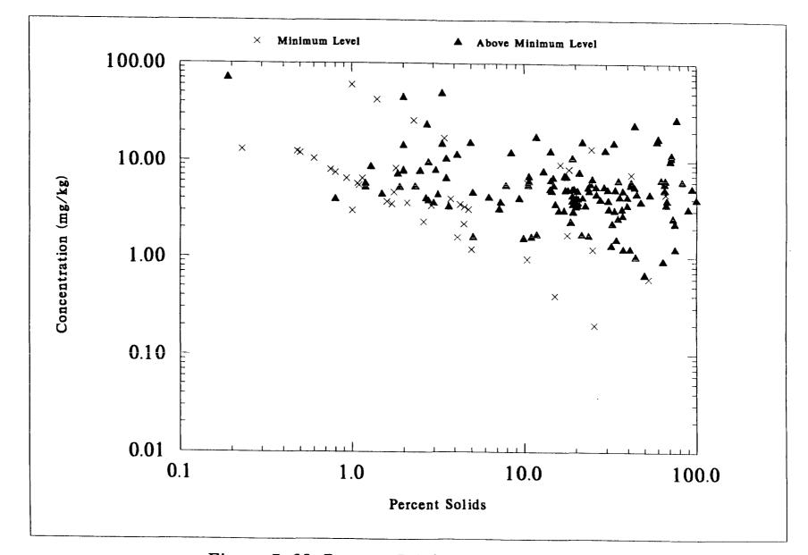
Figure 7-55. Percent Solids of NSSS Samples Versus DRY WEIGHT Concentrations of SELENIUM
