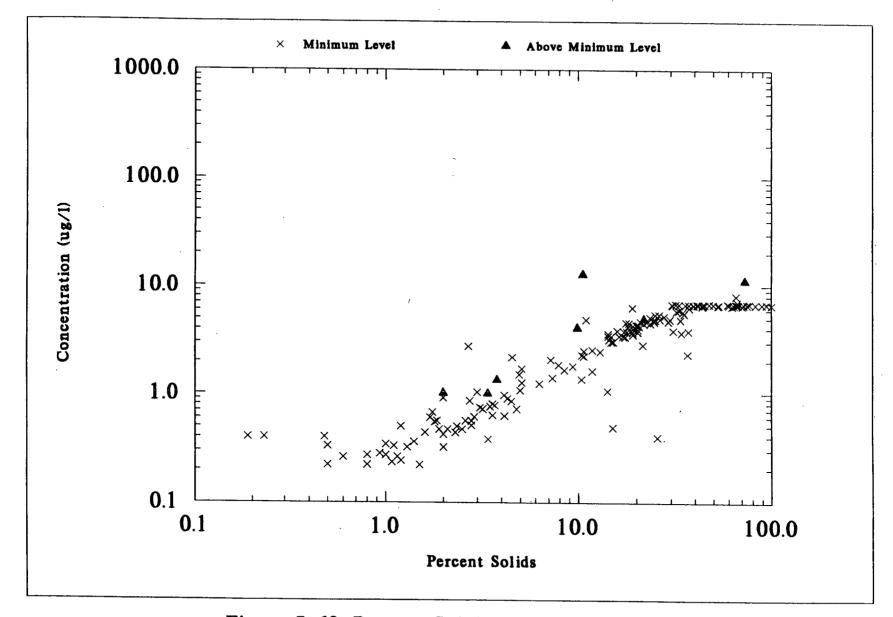
Figure 7-68. Percent Solids of NSSS Samples Versus WET WEIGHT Concentrations of 4.4-DDT
