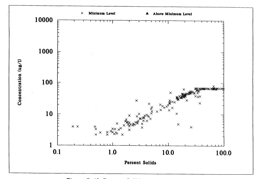
Figure 7-42. Percent Solids of NSSS Samples Versus WET WEIGHT Concentrations of PCB-1016
