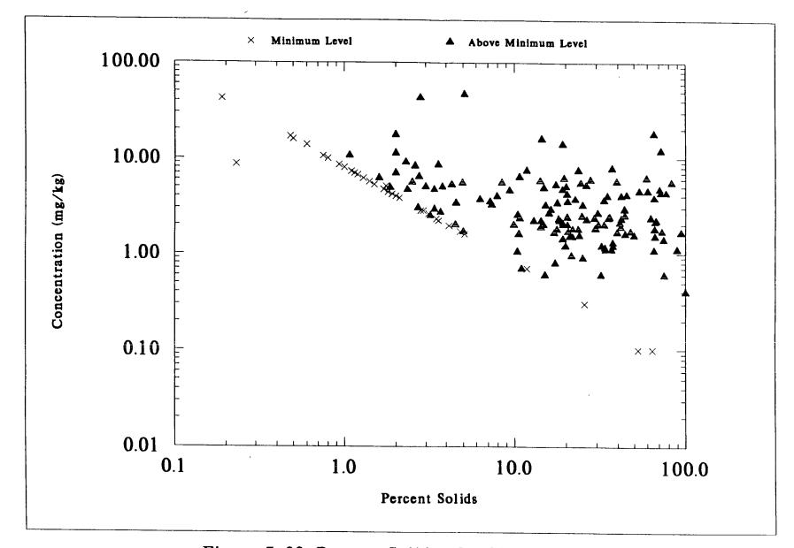
Figure 7-33. Percent Solids of NSSS Samples Versus DRY WEIGHT Concentrations of MERCURY
