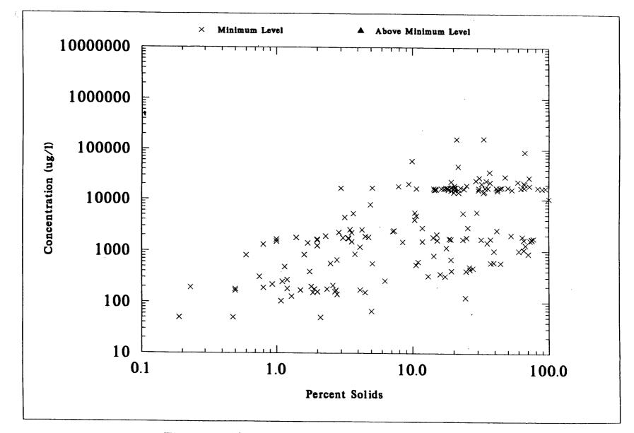
Figure 7-38. Percent Solids of NSSS Samples Versus WET WEIGHT Concentrations of N-NITROSODIMETHYLAMINE
