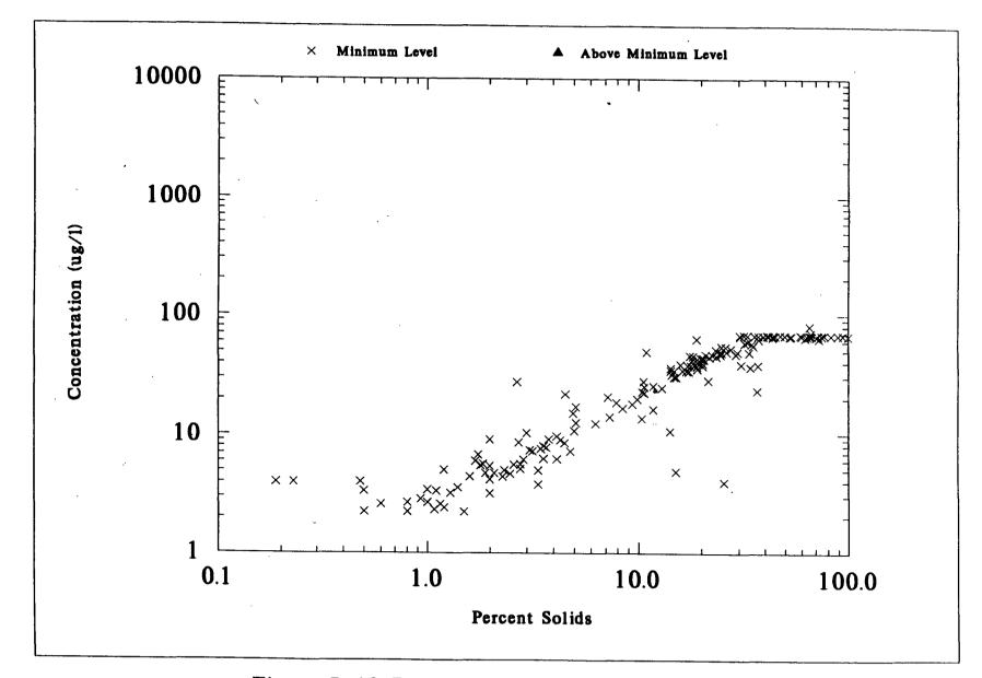
Figure 7-46. Percent Solids of NSSS Samples Versus WET WEIGHT Concentrations of PCB-1232
