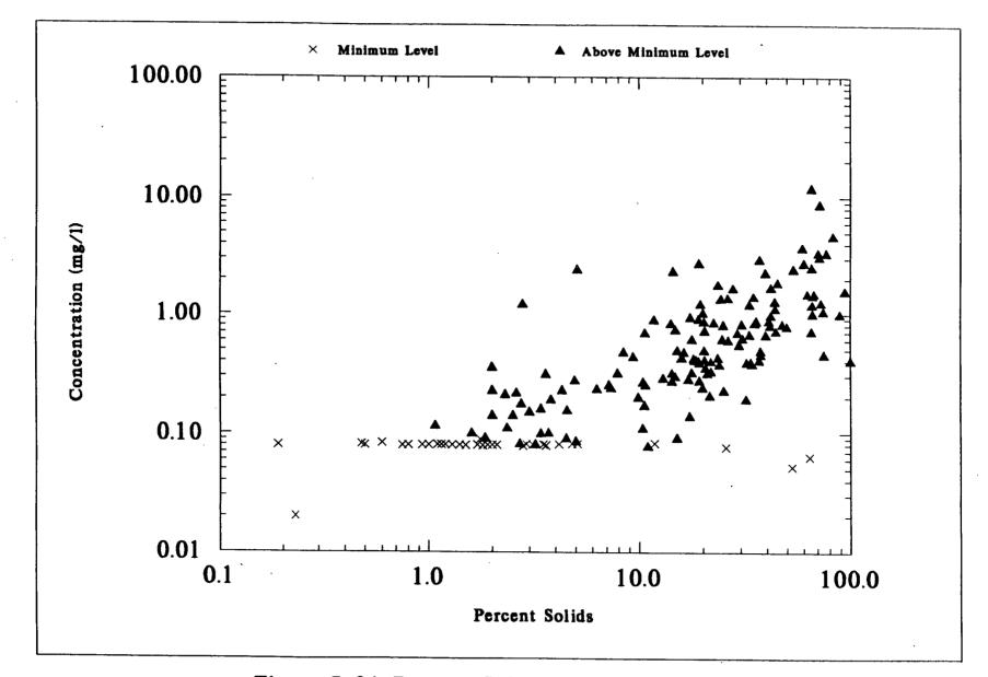
Figure 7-34. Percent Solids of NSSS Samples Versus WET WEIGHT Concentrations of MERCURY
