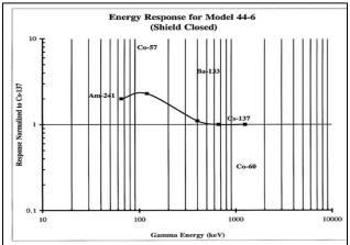
FIGURE 1 – Halogen-Quenched GM Detector Response to Gamma Radiation (A) with Shield Open (B) with Shield Closed
