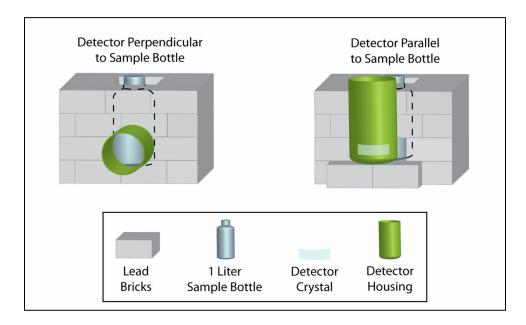
FIGURE 3 - Shown Without Bricks Covering Top of Shielded Geometry. Nal(TI) Detector Example
