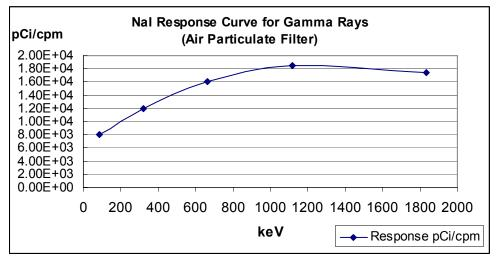
FIGURE 8 – Gamma Energy Response Curve for a NaI(TI) Detector
