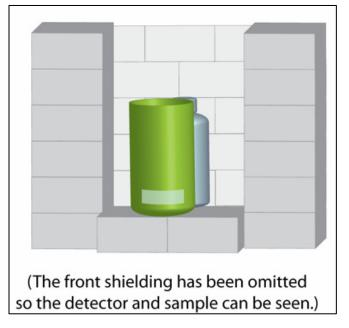
FIGURE 4 – An Improved Orientation for Shielding.
