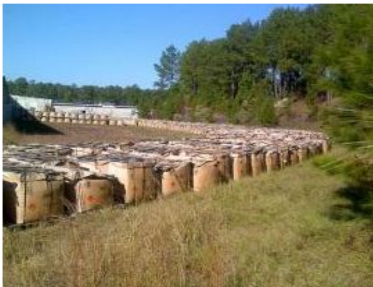
Photo 1: M6 Propellant improperly stored outside by Explo
